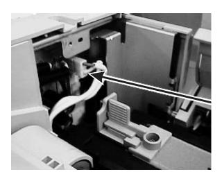
5. Remove the 3 black fuser mounting screws.
