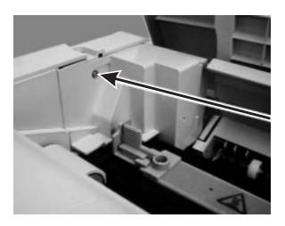
3. Push the latch to lift the top cover, remove the 5 black mounting screws and remove the top cover.
