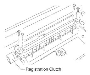
When you reassemble, put conductive grease on the contact portion between the shaft of the registration roll unit and registration roller ground plate.
