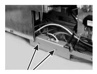
4. Remove the HDRV board from the HK bracket, (2 screws).
