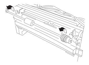
4. Remove the E-ring and MPF clutch.
