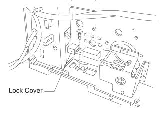
4. Remove the 6 outside mounting screws and 2 screws from inside the frame. Remove drive 1.
