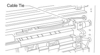
10. Press and slide the paper cassette support plate and remove the paper feed base, (4 screws).
