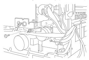
4. Remove the FUD solenoid from the mounting bracket stay, (2 black screws).
