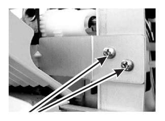
3. Remove the left MPF plate, (2 screws).
