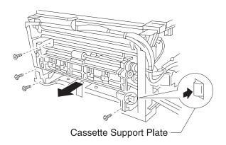
11. Remove the turn guide, (4 screws).
