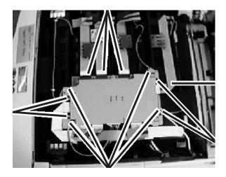
8. Remove the head controller board from the mounting board, (6 screws.)
