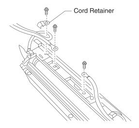
4. Remove the left heater plate from the left side.
