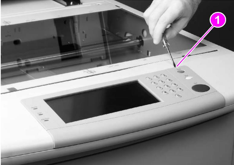
**Figure 62.** Control panel (1 of 3)
