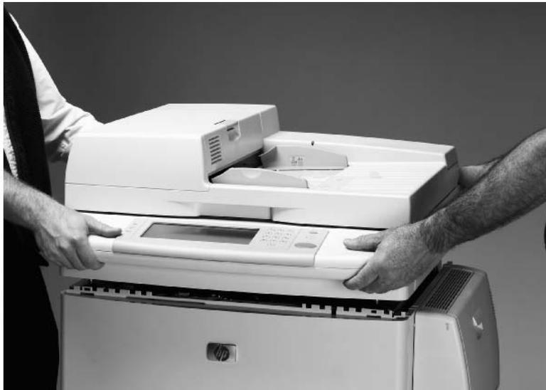
**Figure 191.** Scan engine (6 of 7)
