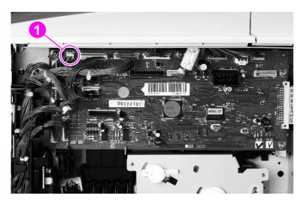
Figure 103. Removing the cartridge fan (1 of 2)
