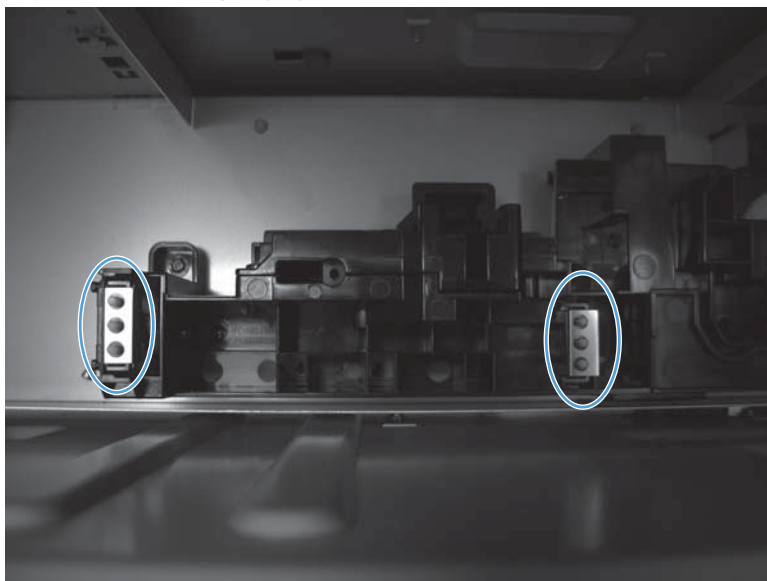
Figure 2-27 Tray 4 paper size switches
