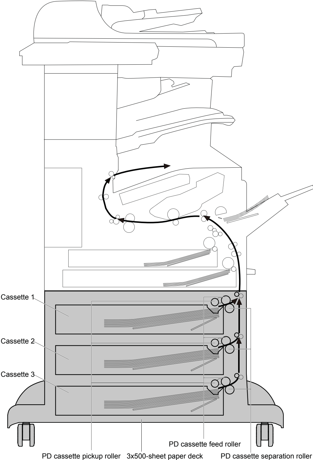
Figure 1-48 Paper deck paper path
