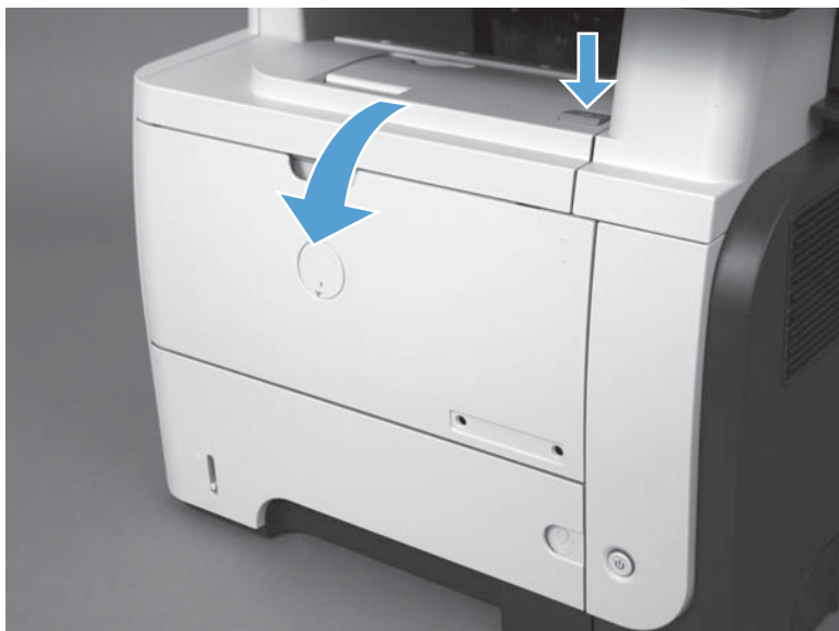
Figure 1-5 Remove the toner cartridge (1 of 2)
