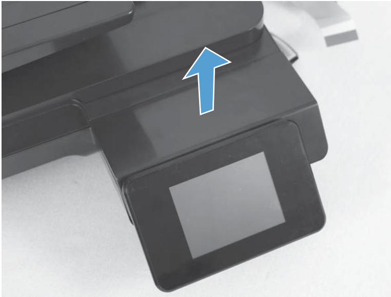
Figure 1-78 Remove the control-panel top-cover (2 of 2)
