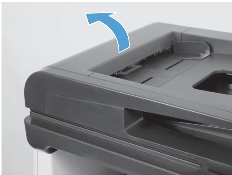
Figure 1-12 Remove the document feeder separation pad (1 of 2)
