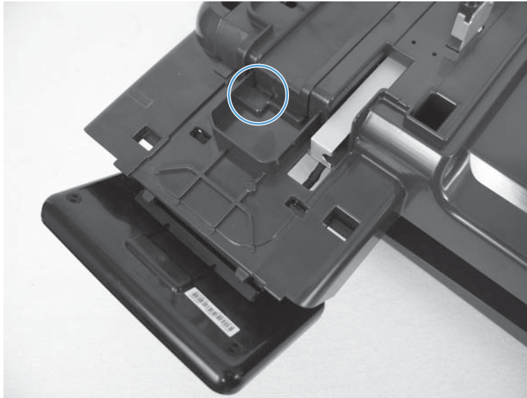
Figure 1-87 Remove the control-panel FFC (3 of 6)
