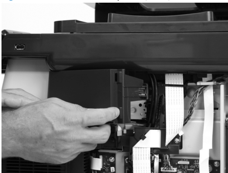
Figure 1-23 Remove the dummy cover (2 of 2)
