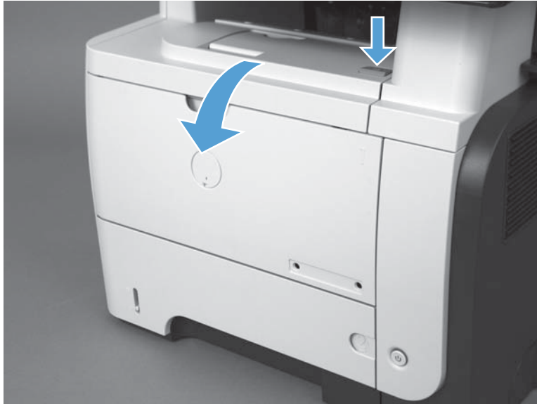
Figure 1-105 Remove the Tray 1 separation pad (1 of 2)
