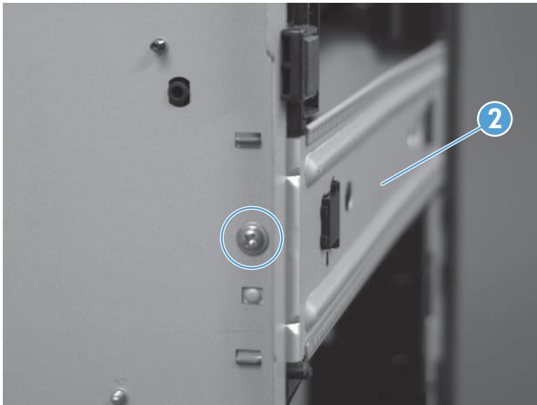
Figure 1-194 Remove the HVPS (2 of 12)
