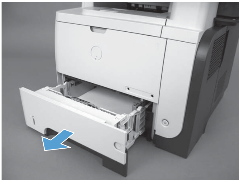
Figure 1-7 Remove the tray
