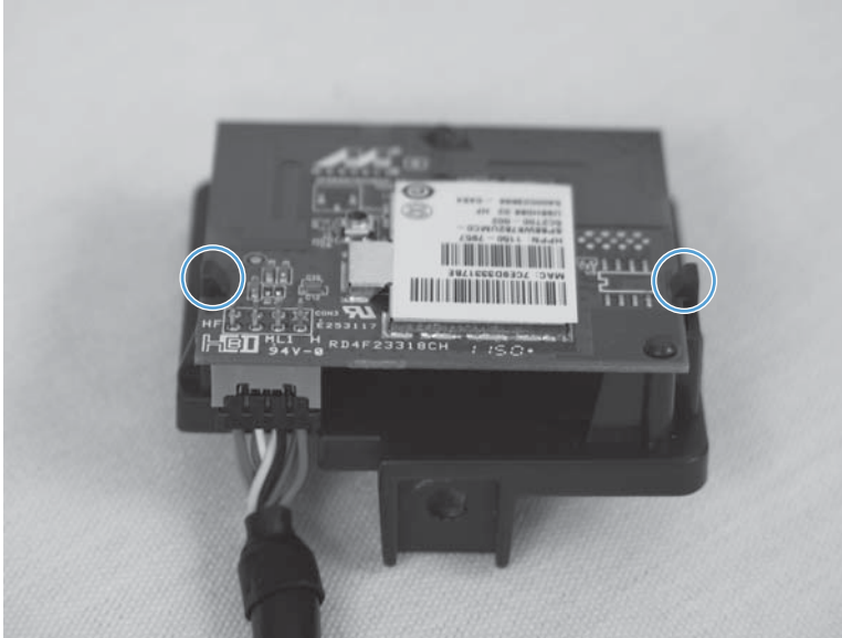
Figure 1-101 Remove the Wi-Fi module and cable (5 of 6)
