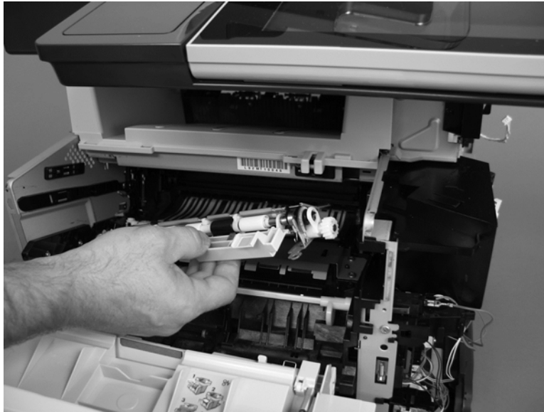
Figure 1-127 Removing the registration roller assembly (3 of 3)
