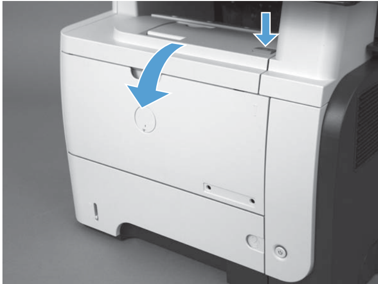
Figure 1-103 Remove the Tray 1 pickup roller (1 of 2)
