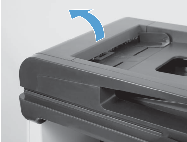
Figure 1-10 Remove the document feeder separation roller (1 of 2)
