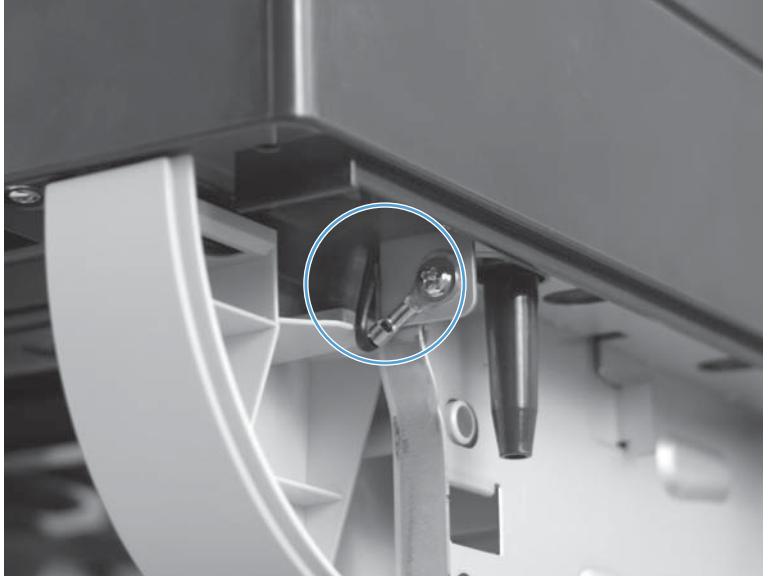
Figure 1-68 Reinstall the document feeder/scanner assembly (3 of 3)
