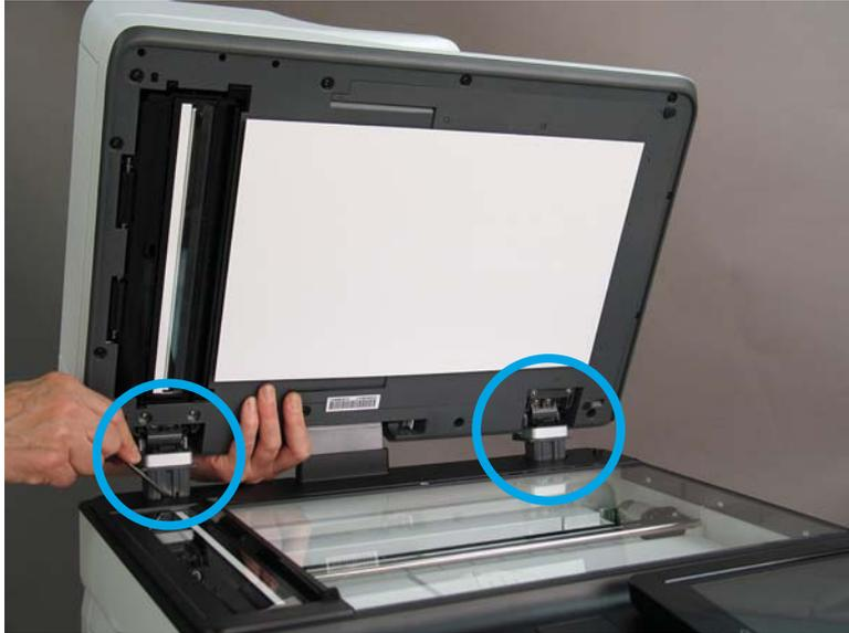
19. Lift the ADF up and remove it.
