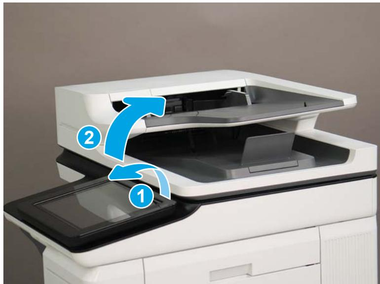
2. Beginning at the right side of the control-panel cover, carefully release five tabs along the top edge of the cover.
