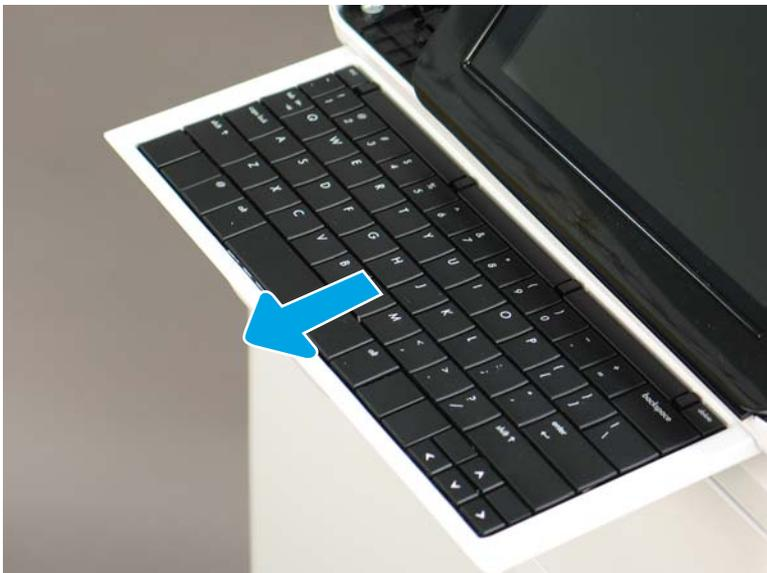
6. Push up on the keyboard tray to release two tabs on the bottom of the tray, and then slide the tray toward you to disengage the tabs.
