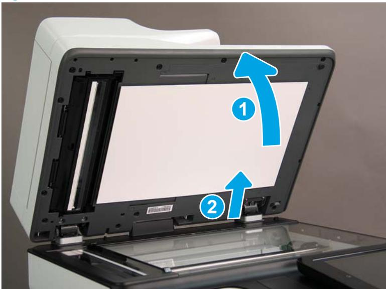
18. Support the ADF, and then use a small, flat-blade screwdriver to release two tabs on the ADF hinges.
