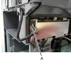
Reseat the flatbed CCD Go to step 3. cable.
