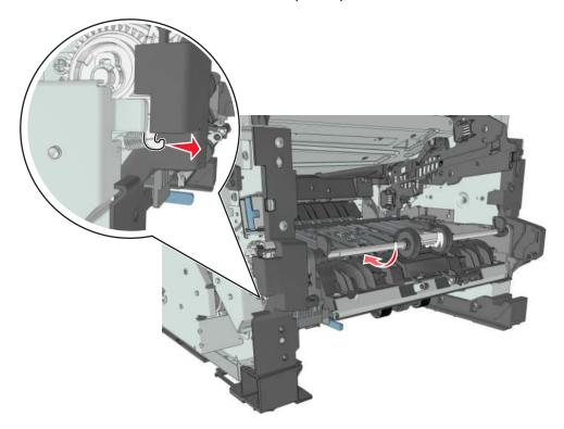
Release the front guide from the guides at each end.
