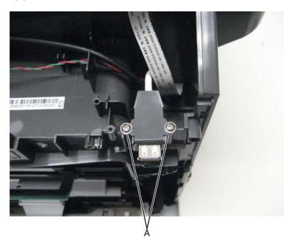
**3** Remove the USB cable bracket.
