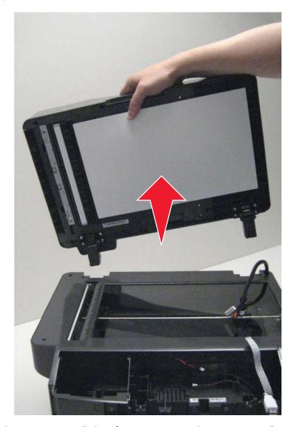
**Installation note:** After the new ADF is installed, perform scanner manual registration, see **"Scanner manual registration"** on page 178 and scanner calibration, see **"Scanner calibration"** on page 155.
