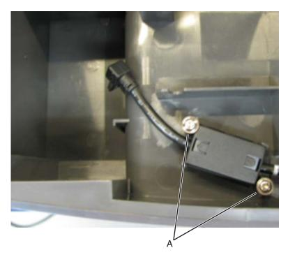
**9** Feed the wireless cable through the channel on the left side of the printer.
