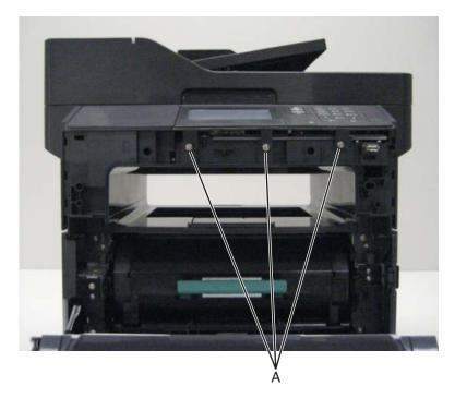
4 Lift the control panel assembly, disconnect the ribbon cable (JUICC1) from the UICC card, and then feed the ribbon cable through the wire channel.
