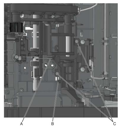
Below is the image of the cam release and bracket.
