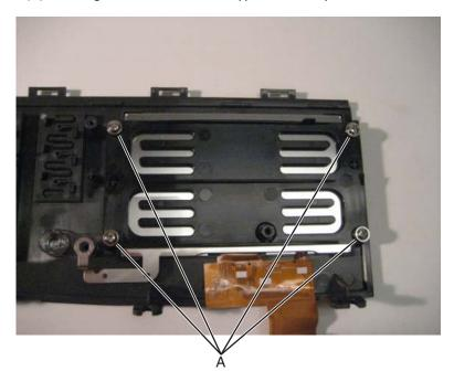
4 Remove the ground shield.
