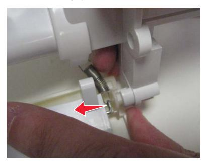
5 Slide the tray to the right, and remove the MPF tray and spring.
