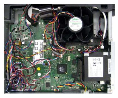
7 Disconnect the two cables (A) from the RIP board.
