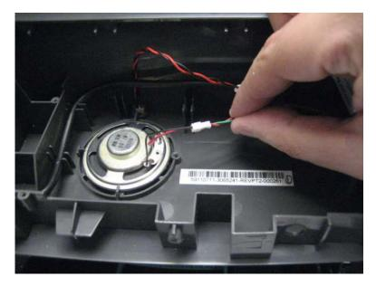
**9** Feed the speaker cable through the channel on the right side of the printer.
