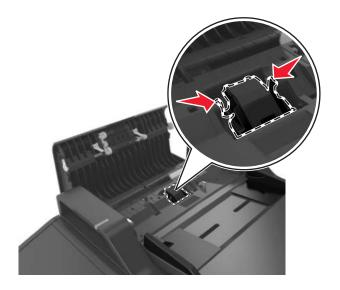
Pull away the separator pad and remove.
