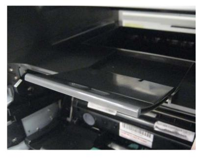
2 Push up on the center tab of the bin extender while pulling the extender towards the front of the printer.
