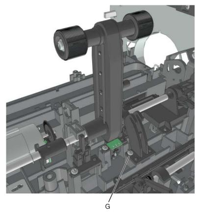
17 Remove the ACM assembly with shaft.Below is the ACM assembly with media present sensor flag and bracket.
