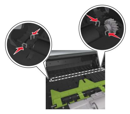
**2** Lift to remove the transfer roll.
