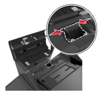
Pull away the separator roll and remove.
