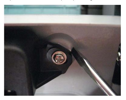
**5** Remove the three screws (B) securing the LSU.
