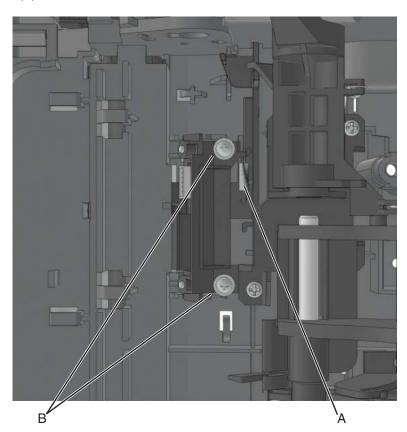
**9** Disconnect the cable from the sensor.
