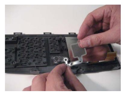
**5** Remove the light tube (B).
