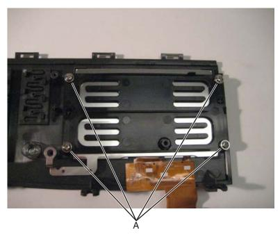
4 Remove the ground shield.
