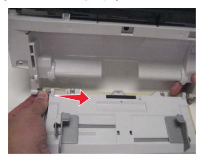
**Installation note:** Insert the straight end of the spring into the hole on the front access cover before sliding the MPF tray onto the left pivot of the front access cover.
