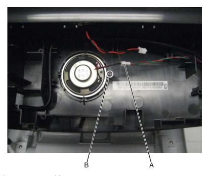
Slide the speaker off the scanner assembly.
