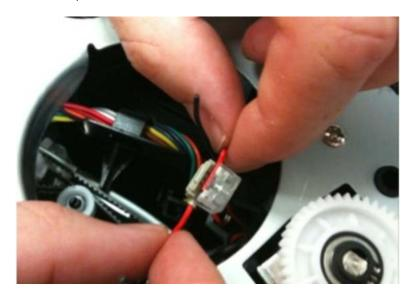
**g** Squeeze the IDC to partially lock the wires in place, and then use a pair of pliers to crimp the IDC.
