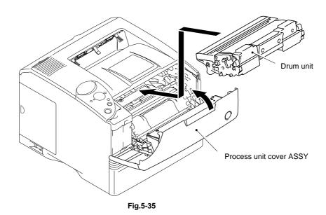
5) Install the drum unit into the printer and close the process unit cover ASSY.
