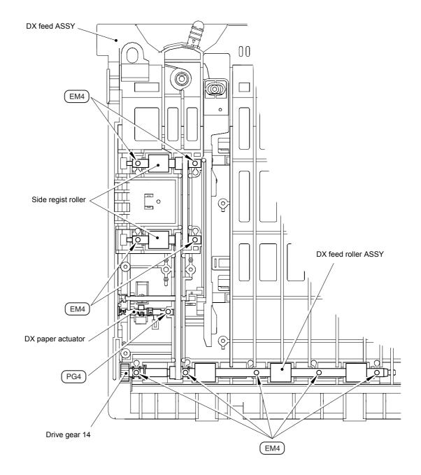
EM4: Grease EM-D110 4mm dia. ball PG4: Grease PG-662Y 4mm dia. ball
