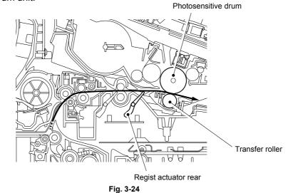
The regist rear actuator in the path from the feed roller to the transfer roller controls the first print position on the paper.
