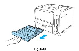
(5) Pull the jammed paper out of the printer.
