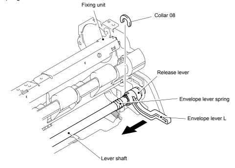
(28) Remove the collar 8, and move the release lever, the envelope lever L, and the envelope lever spring toward inside.
