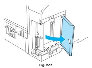
(4) Loosen the two screws, and then remove the Network cover plate.
