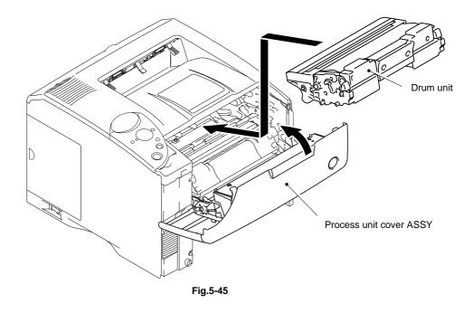
8) Install the drum unit into the printer and close the process unit cover ASSY.
