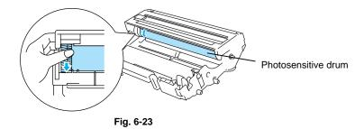
(3) Wipe the surface of the photosensitive drum with a cotton swab until the dust or paper powder on the surface comes off.
