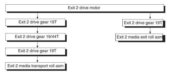
The transmitted driving force drives the exit 2 media transport roll assembly and the exit 2 media exit roll assembly through the gears.
