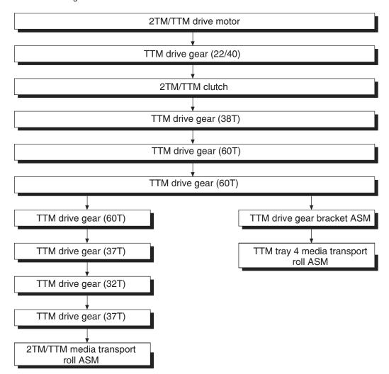
The driving force transmitted to the gear 22/40T drives the transport roll assembly through the clutch and gears.
