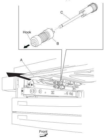
Note: Before re-installing, do not touch the rubber surface of the pick roll (B).
