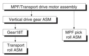
The MPF/transport drive motor provides the driving force transmitted to the gear drives, the transport roll assembly, and the multipurpose feeder (MPF) pick roll.
