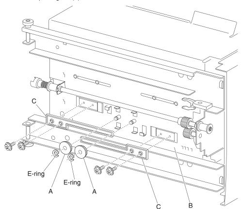
5. Remove four screws securing the two rack gears (C) to the frame assembly (B).
