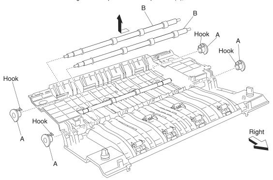
Note: When replacing the two duplex media transport rolls (B), do not touch the rubber surface.
