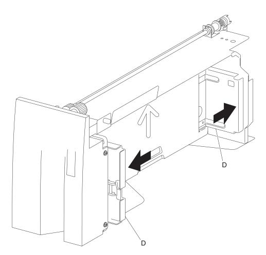
Note: Before re-installing, move the two side guides (D) of the frame assembly (B) fully outward before installing the two pinion gears (A).
