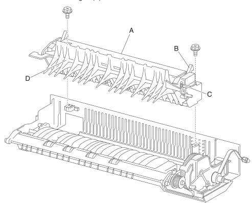
Note: After reinstalling the upper guide assembly (A), ensure the exit 2 access handle (B) operates freely.
