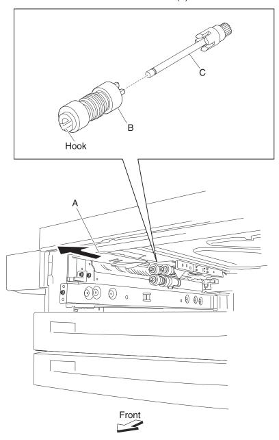
Note: Before re-installing, do not touch the rubber surface of the feed roll (B).
