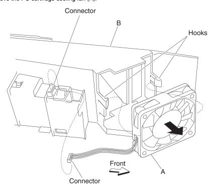
Note: Before reinstalling the PC cartridge cooling fan (A), ensure the fan blade is facing toward the front of the machine.
