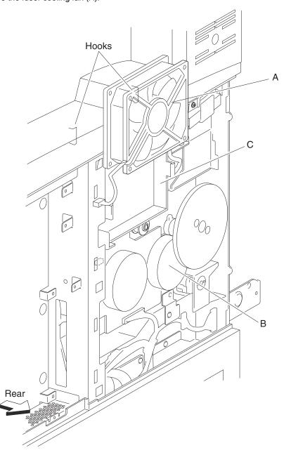
Note: Before reinstalling, the fuser cooling fan (A) must be installed with the center label facing outward.
