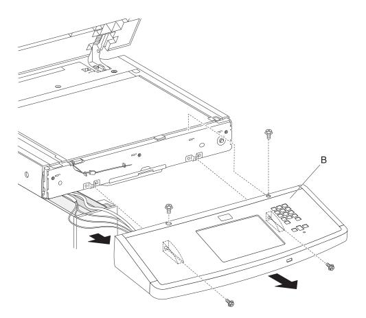
10. Guide the operator panel cable and the USB-Smart card-LED cable assembly through the rear of the printer so that they can be pulled through from the front.
