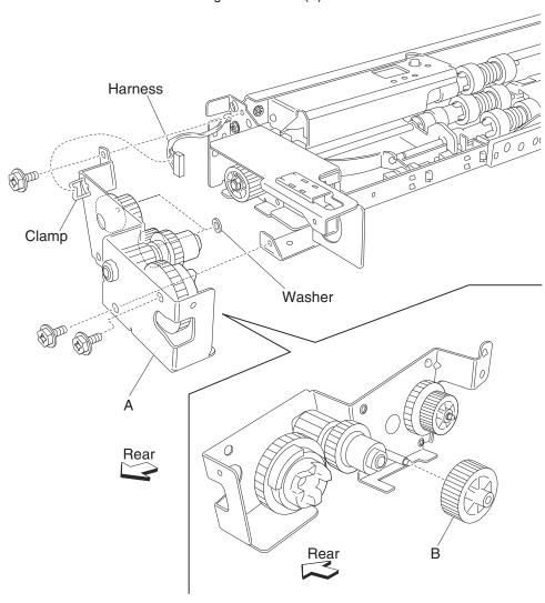
**6.** Remove the media feed unit drive gear - 29 tooth (B).
