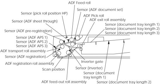
A document sheet set in the document tray assembly is fed through the ADF feed roll, ADF pick roll, and ADF registration roll assembly. The document image is scanned at the scan position, and the document sheet is ejected through the ADF feed-out roll assembly and the ADF exit roll assembly. For a duplex document sheet, the image on side 1 is scanned at the scan position and then the document sheet is inverted and fed to the ADF transport roll assembly again.
