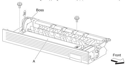
4. Remove the upper guide assembly (A).
