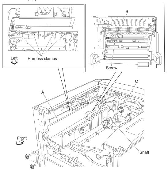
Note: Before reinstalling, ensure the shaft (C) on the toner cartridge guide assembly (A) is inserted into the toner add motor assembly (D).
