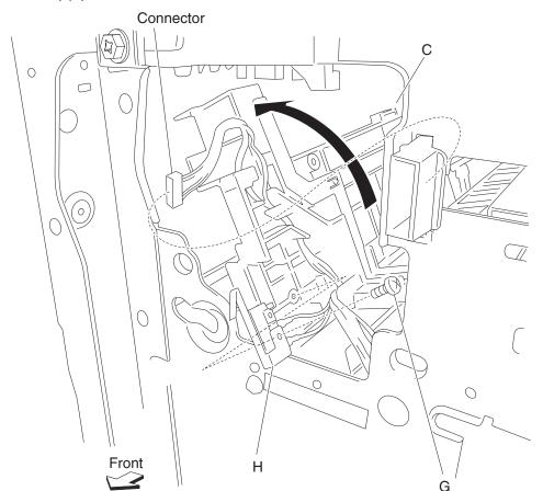
**24.** Remove the PC cartridge guide assembly (C) from the printer.
