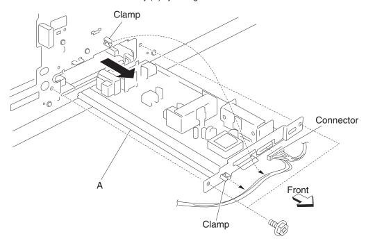
Note: Before reinstalling, ensure the HVPS (A) is inserted into the side slots properly.
