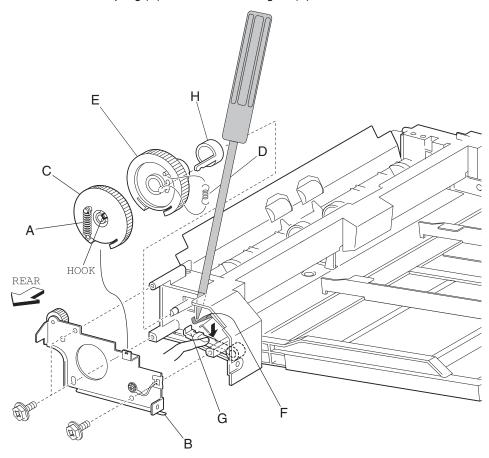
**9.** Remove the drive gear cam (E) and the drive stopper (H).
