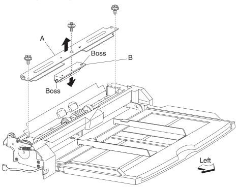
**Note:** Before reinstalling, ensure you do not touch the plastic roll surface.
