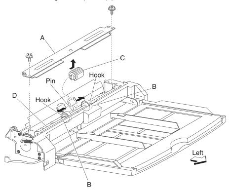
Note: Before reinstalling the MPF pick roll assembly (C), do not touch the rubber surface.
