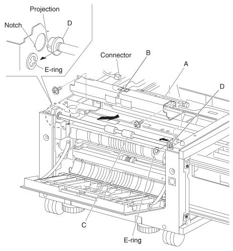
Note: Before re-installing the 2TM/TTM media transport roll assembly (C), do not touch the rubber surface.
