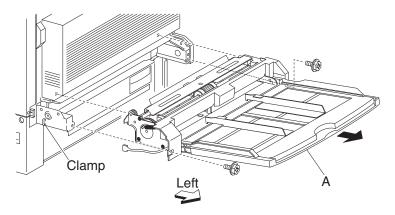
Note: Before reinstalling, place the harness along the slot on the left of the MPF feed unit assembly (A) so it does not pinch the harness between the feed unit.
