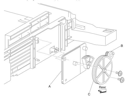
Note: Extra force is required to pull the tray lift coupling gear 13 tooth (B) and the tray lift gear 13/60 tooth (C) from bracket (A).
