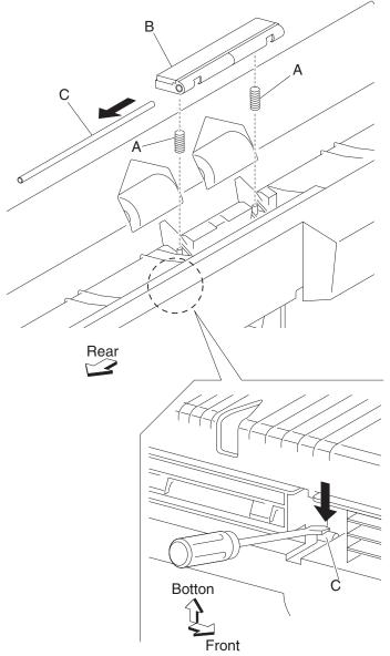
Note: Before reinstalling, ensure the two springs (A) remain in the proper position during reassembly of the feed shaft assembly and MPF feed roll.
