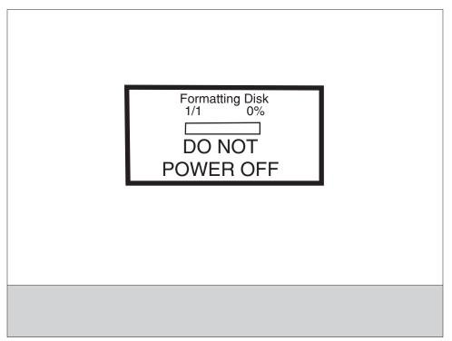
This test cannot be interrupted once it has begun. After the test finishes, either Di sk Test/CI ean Test Passed or Di sk Test/Clean Test Failed appears on the display. Press **Stop** 🔯 to clear the final message and return to DEVICE TESTS.
