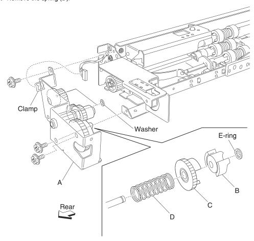
Note: Before reinstalling, ensure all gears and washers attached to bracket (A) are securely installed.
