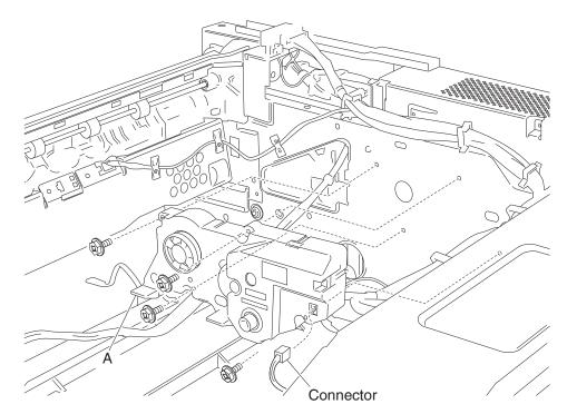
Note: Before reinstalling, ensure the shaft on the toner cartridge guide assembly is inserted into the toner add motor assembly (A).
