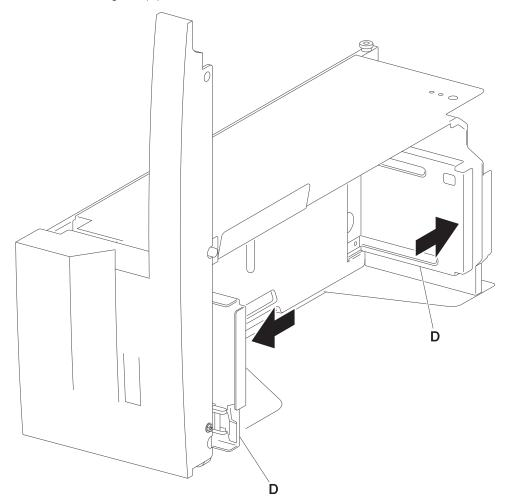
Note: Before re-installing, move the two side guides (D) of the frame assembly (B) fully outward before installing the two pinion gears (A).
