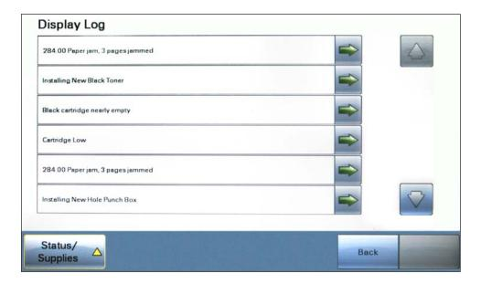
Each logged event is identified by the text that appeared when the event occurred. For instance, if the log recorded a 900 Service Error, the Display Log would show 900 Service RIP Software. Log entries appear in chronological order.
