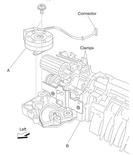
Warning: Before reinstalling, secure the media shift motor (A) harness to the clamps on the exit 1 media shift assembly (B) to prevent damage.
