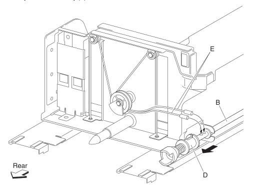
8. Remove the two tray 3 rear cables (E) from the tray lift shaft assembly (B).
