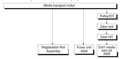
The driving force transmitted to the gear drives the transport roll assembly, multipurpose feeder (MPF) feed roll, registration roll assembly, fuser assembly, and exit 1 media exit roll assembly through the clutch and gears.
