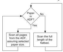
During the test, Running... Flatbed: xxxxx ADF: xxxxx appears on the display. The Flatbed number increases each time the scanner performs a flatbed scan, and the ADF number increases each time the scanner performs an ADF scan.
