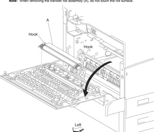
Note: Before reinstalling the transfer roll assembly (A), do not touch the roll surface.
