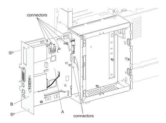
5. Remove the RIP card chassis bracket assembly.
