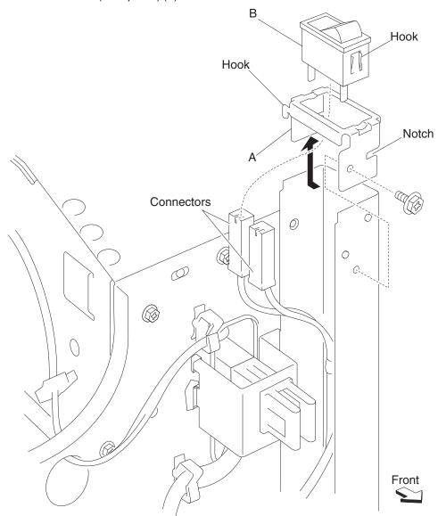
Warning: Before reinstalling, ensure the four connectors are plugged into their proper location to prevent damage.
