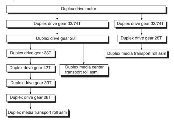
The transmitted driving force drives the two duplex media transport roll assemblies, and the (duplex media center transport roll assembly) through the gears.
