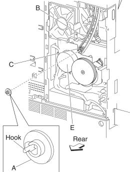
Note: Press on the exit 1 drive belt (B) while slowly turning the motor (E) by hand.
