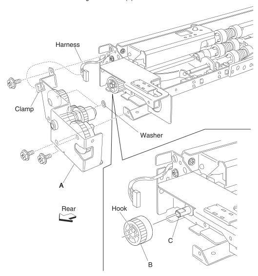
Note: Before re-installing, ensure all gears and washers are securely attached to the bracket (A).
