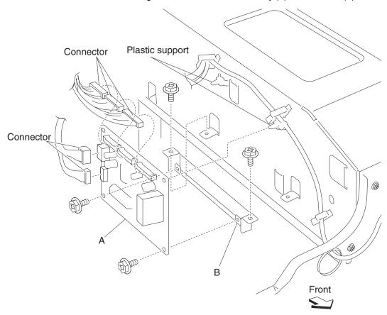
7. Remove the exit 2 card assembly (A).
