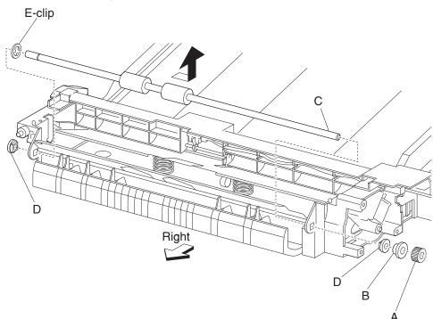
Note: Before reinstalling the MPF transport roll assembly (C), do not touch the rubber surface.
