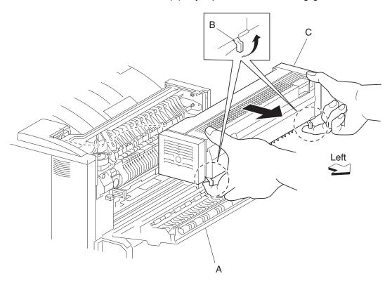
Note: Before reinstalling, ensure the exit 2 (C) unit is properly aligned and the electrical connector is properly connected.
