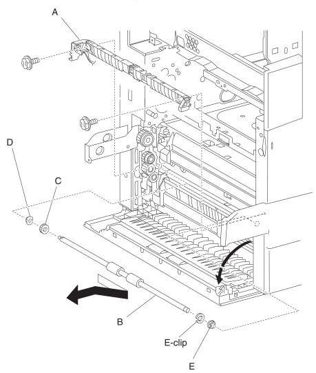
Note: Before reinstalling the media transport roll assembly (B), do not touch the rubber surface.
