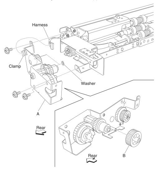
Note: Before re-installing, ensure all gears and washers are securely attached to the bracket (A).
