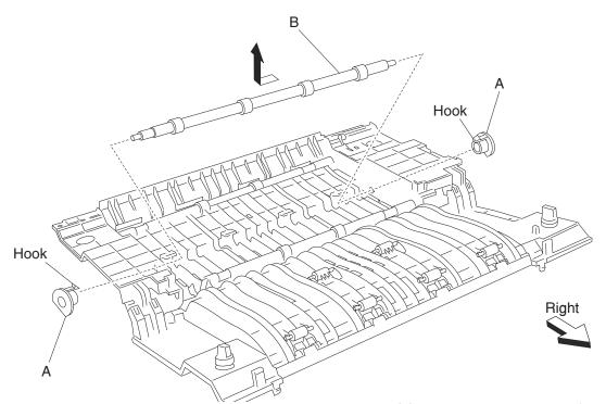
Note: When replacing the duplex media center transport roll (B), do not touch the rubber surface.
