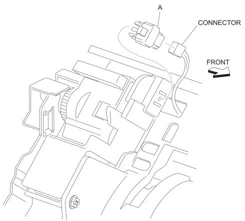
Note: Before reinstalling the switch (exit 2 left door interlock) (A), ensure all the harnesses and connectors are properly installed.
