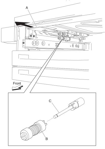
Note: Before re-installing, do not touch the rubber surface of the separation roll (B).
