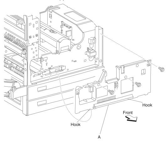
Note: To reinstall the front inner cover (A), start with the four plastic hooks on the bottom of the front inner cover.
