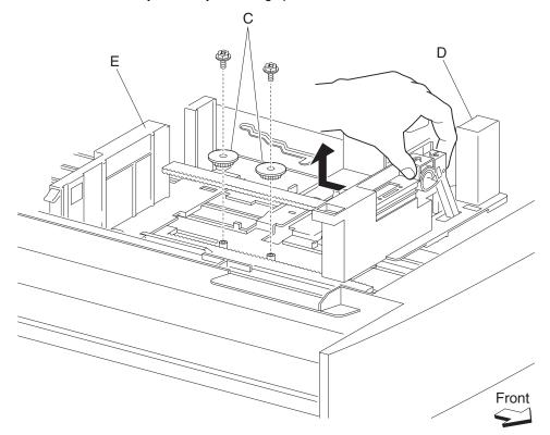
Note: Before reinstalling the pinion gears (C), slide the front media tray guide assembly (D) and the rear
