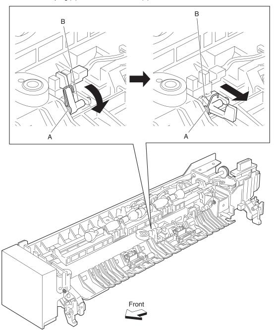
Note: Before reinstalling the exit 2 actuator (B), ensure the spring (A) is properly installed.
