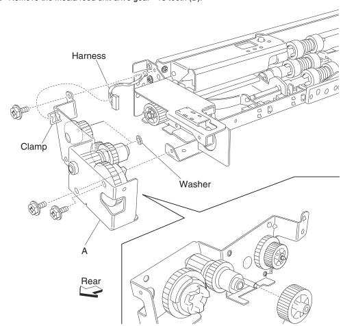
Note: Before reinstalling, ensure all gears and washers are securely attached to the bracket (A).
