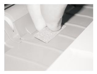
**Note:** To avoid jams, in the ADF, ensure the leading edge of the pick pad is pressed firmly into the guide.
