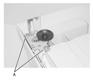
12. Lift to remove the flatbed motor.
