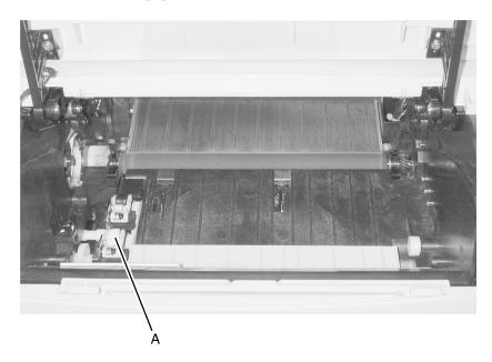
When a reference plate (reference edge) assembly is removed, reinstallation requires alignment. Use a long shank (6-inch) Phillips screwdriver to adjust the rear screw holding the assembly in place. It is accessed through the hole in the main drive assembly between the RIP card cage and the main motor PCB. Adjusting the screw counterclockwise rotates paper counterclockwise in the MFP path.
