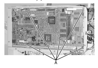
6. Remove one screw above the USB connector.
