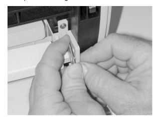
4. Support the left side with the left hand while separating the left hinge.
