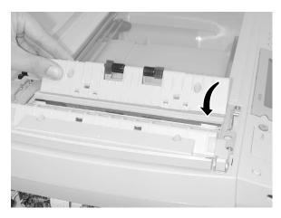
**Note:** Reinstall: ensure extended edge of the R2 idler **[A]** is slipped under the scanner glass.
