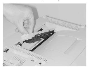
6. Carefully, lift the rear edge of the top cover to clear the exit flags and rotate the front cover hinge until the cover is in a vertical position.
