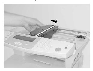
**Warning:** Do not touch the two lamps on top of the unit. This could shorten the life of the lamps.
