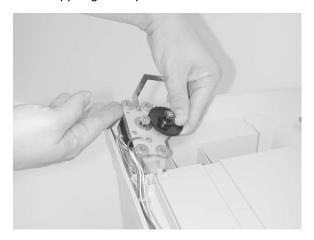
**Note:** This plate needs to be attached to the new flatbed motor.
