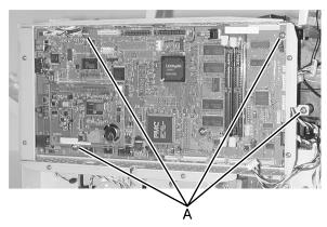
8. Gently pull the bottom of the cage out and lift up off the two posts at the top.
