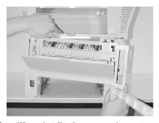
**Note:** When reinstalling the rear cover, be sure to position the fuser exit guide fingers such that they are not bound by the rear cover. If a bind occurs, a jam occurs.
