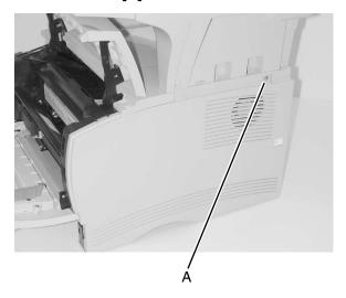
5. While pulling out on the top of the right side cover, use your left hand to release the two latches (top front [A] and lower front [B]).
