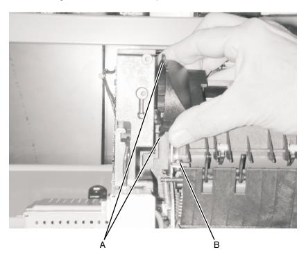
Unplug the exit sensor, and thermistor connector [A].
