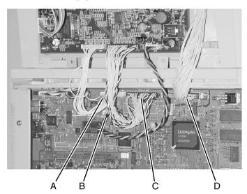
**Warning:** When feeding cables through the RIP cage, take care not to strip the insulation from the cables. This could result in a short.
