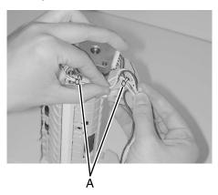
3. Remove the three screws [A] that fasten the ADF motor assembly to the ADF feeder assembly.
