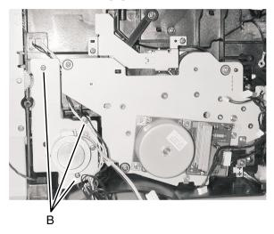
5. Lift the stepper motor out.
