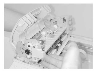
4. Use a screwdriver to release 2 tabs [A].
