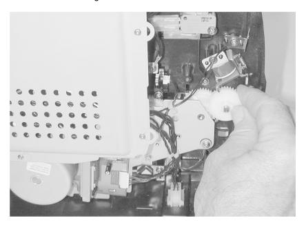
7. Remove two screws [A] holding the roller assembly and one screw facing the front of the printer.
