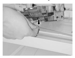
12. Remove the CCD carriage.
