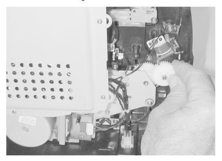
4. Remove the gear train assembly. See "Main drive assembly removal" on page 4-44 for more information.
