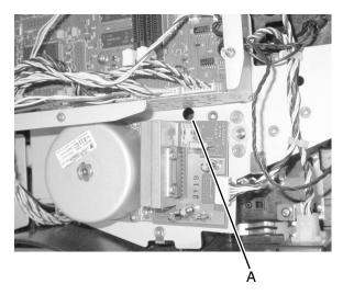
When a reference plate (reference edge) assembly is removed, it requires alignment. Use a long shank (6–inch) Phillips screwdriver to adjust the rear screw holding the assembly in place. It is accessed through the hole in the main drive assembly [A], located between the RIP card cage and the main motor PCB. Adjust the screw counterclockwise which rotates paper counterclockwise in the MFP path (image clockwise) and vice versa.
