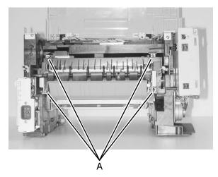
11. While pulling the exit guide down, gently start pulling the fuser towards you, unplugging the fuser lamp [A].
