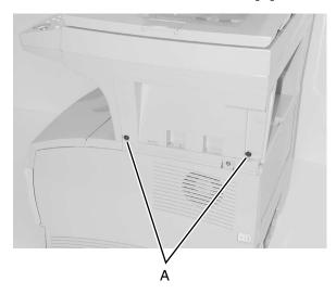
4. From the rear of the scanner, slide the left scanner cover to the rear and remove.
