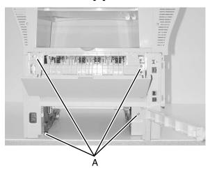
8. For better leverage, move the machine to the edge of the table. Lift the top cover slightly with one hand while pulling out on the rear cover.
