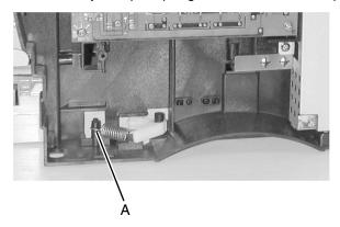
3. Rotate the lever counterclockwise as far as possible and lift out.
