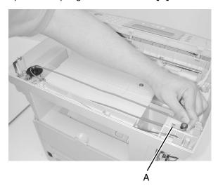
7. Lift the timing belt off the gears to remove.
