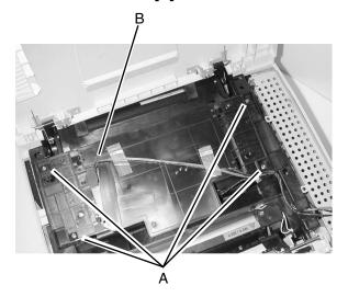
**Note:** Mark alignment of the printhead at the screw areas with the printhead to keep the same alignment upon reinstallation.
