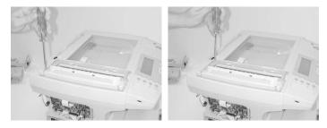
8. Pull idler and bracket away from scanner and remove.
