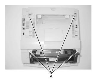
5. Remove the duct assembly in the top cover.
