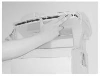
2. Lift the front of the operator panel to release pivots in the rear.
