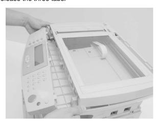
9. Lift the scanner cover, and thread cable through chimney to remove.
