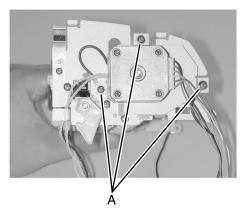
Carefully remove the ADF motor assembly from the ADF feder assembly. Ensure the gears on the ADF assembly remain in the uint.
