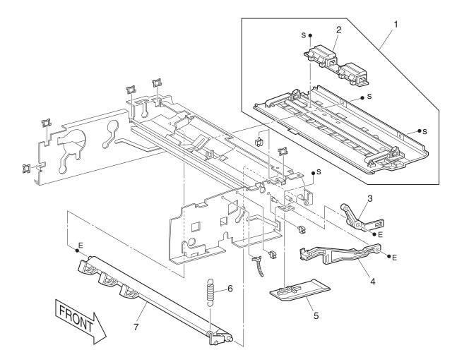
Assembly 4: DADF Separator Pad Asm. and Paper Stop
