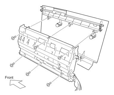
When replacing the jam access door lever, align the key with the keyway in the lower cover as shown.
