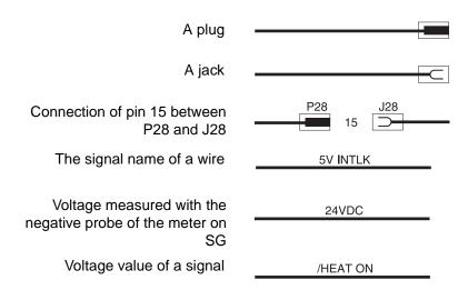
/ = The voltage goes LOW when the signal is ON.
