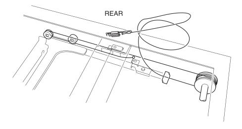
**18.** Engage the cable assembly-scan, rear to the pulley-idler.
