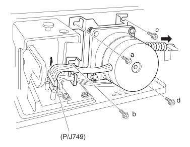
In replacing the scanner motor assembly, secure it with the screws aligned with the marked positions.
