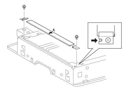
When reinstalling the DADF platen glass place, ensure the white stripe on the glass is positioned toward the rear of the scanner.
