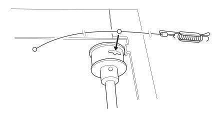
**12.** Wind the spring-exit hooking side of the cable assembly-scan, rear around the pulley-capstan, rear by 1.5 turns.
