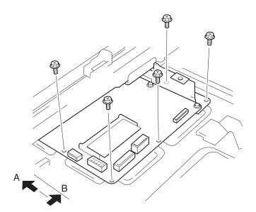
**10.**Remove the scanner system card.
