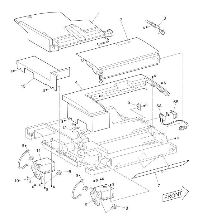
Assembly 2: DADF Cover, Switch, and Hinge (Rear)
