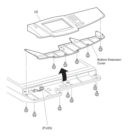
**Note:** When replacing the user interface panel, ensure the DIP switches on the bottom of the user interface panel are set correctly. Position 1 and 2 should be **On**, while the other positions are set to **Off**.
