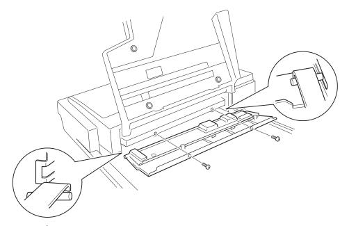
**4.** Remove the screw and slide the separator pad assembly toward the front, and raise to remove it.
