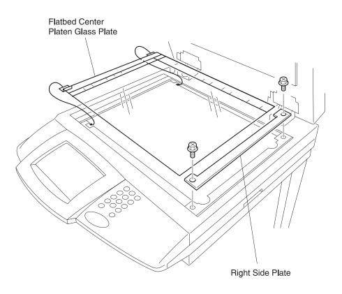
When replacing the flatbed center platen glass plate:
