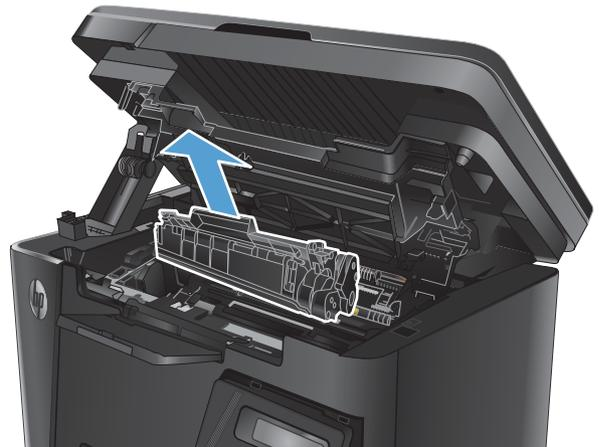
4. Remove any jammed paper from the toner-cartridge area. Use both hands to remove jammed paper to avoid tearing the paper.
