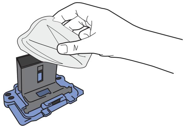
13. Insert the notches on the separation pad assembly into the slots on the bottom of the product.
