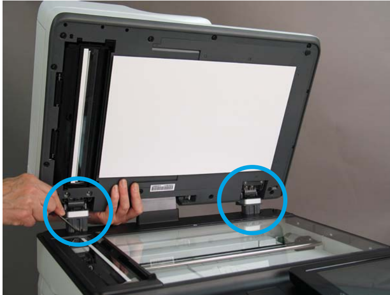
Figure 1-1107 Release two tabs on the ADF
