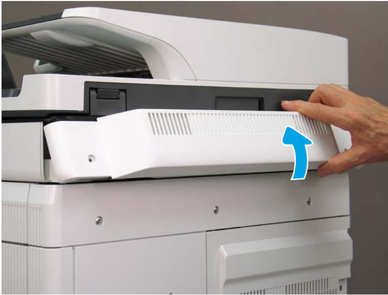
Figure 1-1101 Remove the image scanner back cover
