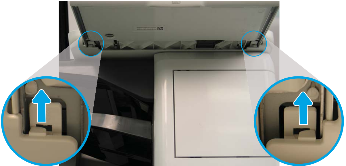
Figure 1-1182 Release two tabs
