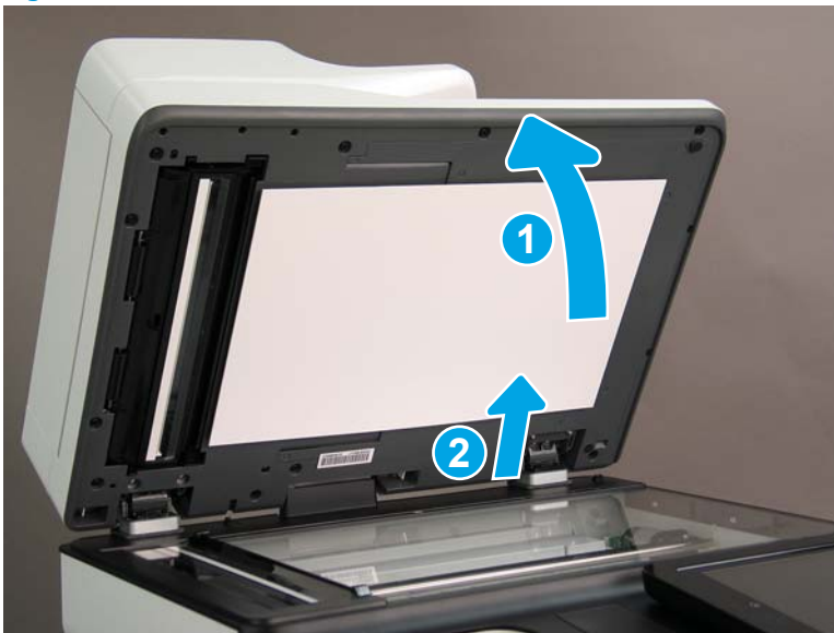
Figure 1-1106 Tilt and lift the ADF
