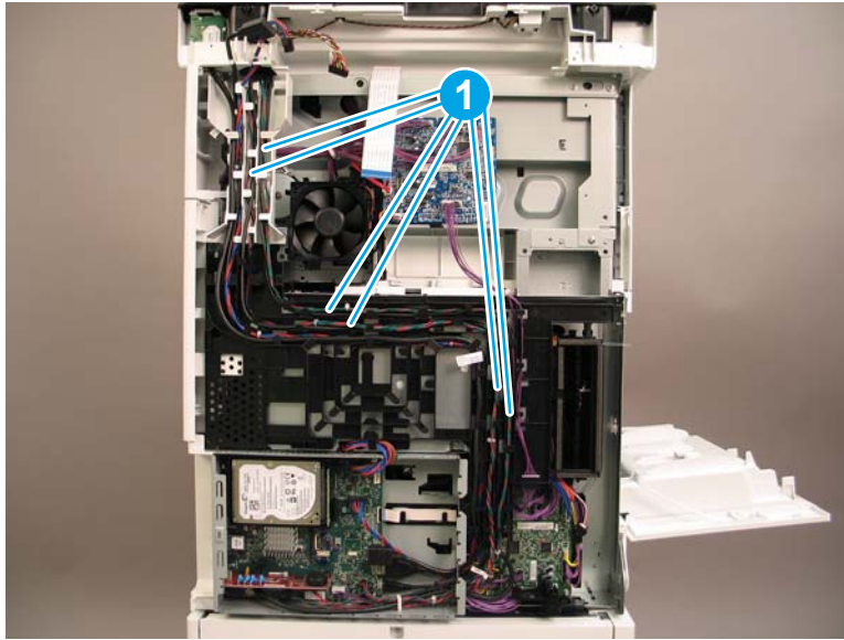
Figure 1-1203 Release the formatter cables
