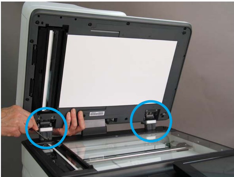
Figure 1-1194 Release two tabs on the ADF
