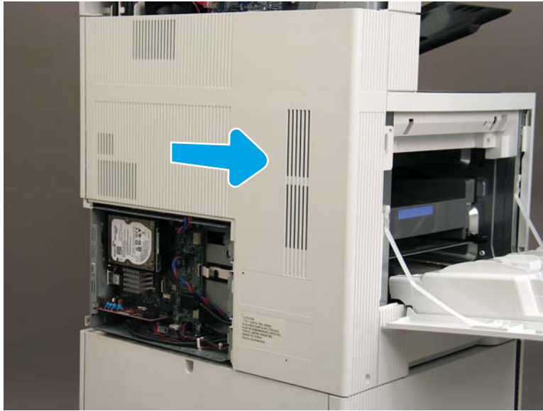
Figure 1-1199 Slide the rear cover
