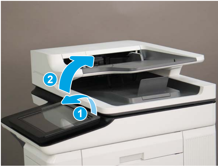
Figure 1-1177 Tilt the control panel and open the document feeder
