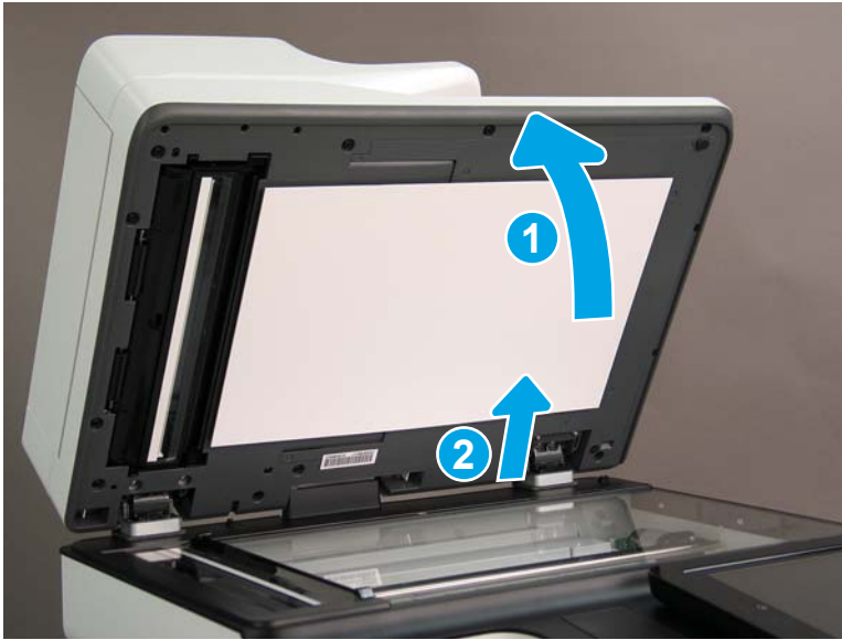
Figure 1-1193 Tilt and lift the ADF
