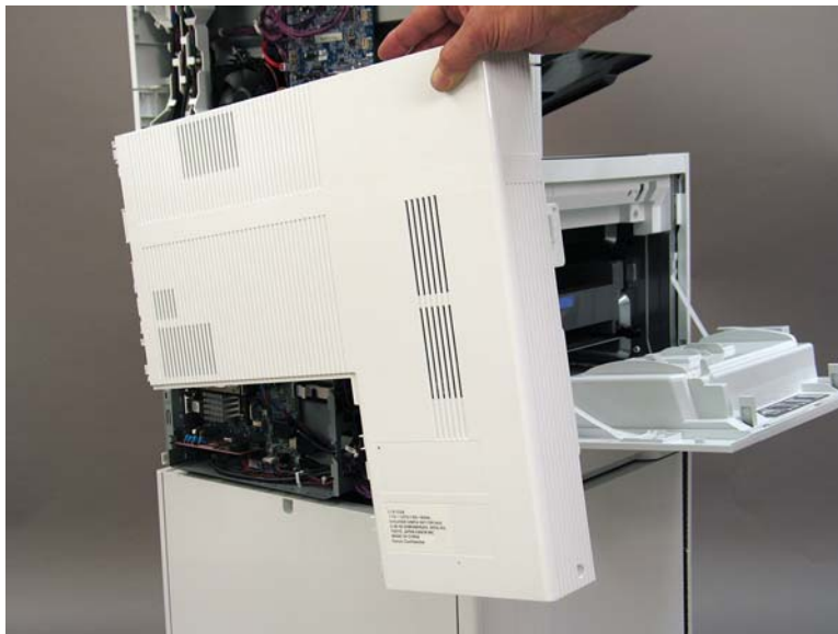
Figure 1-1200 Remove the rear cover
