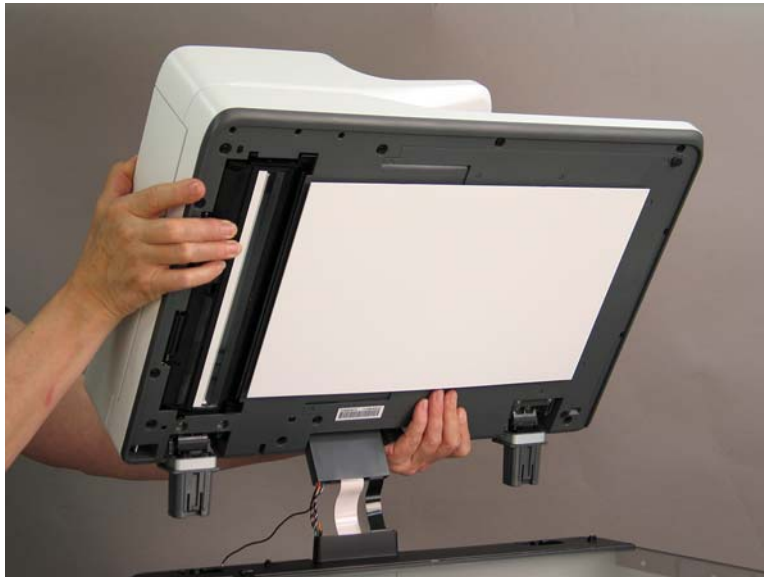
Figure 1-1108 Lift and remove the ADF
