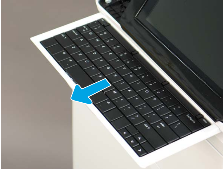
Figure 1-1181 Slide the keyboard tray out
