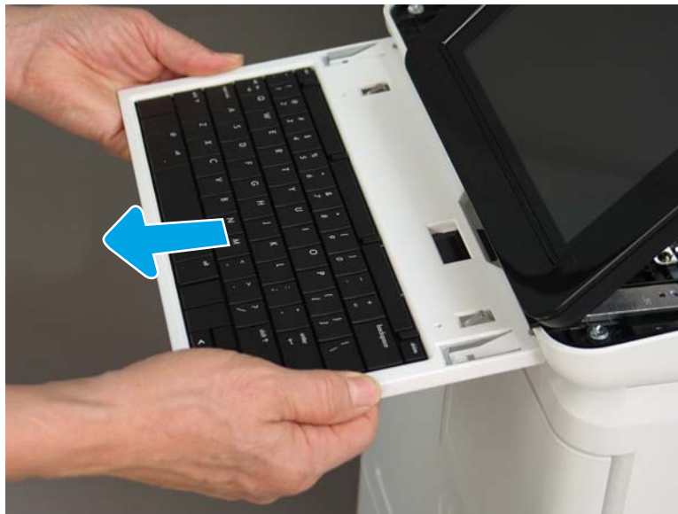
Figure 1-1096 Remove the keyboard
