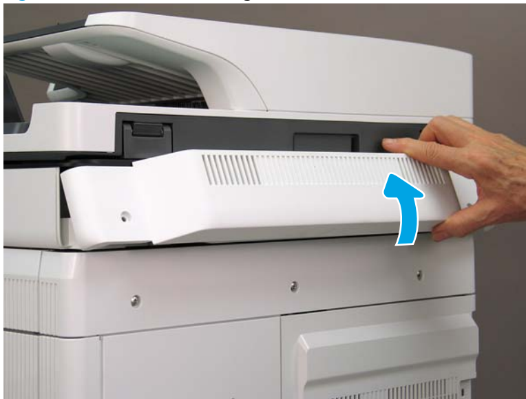
Figure 1-1188 Remove the image scanner back cover
