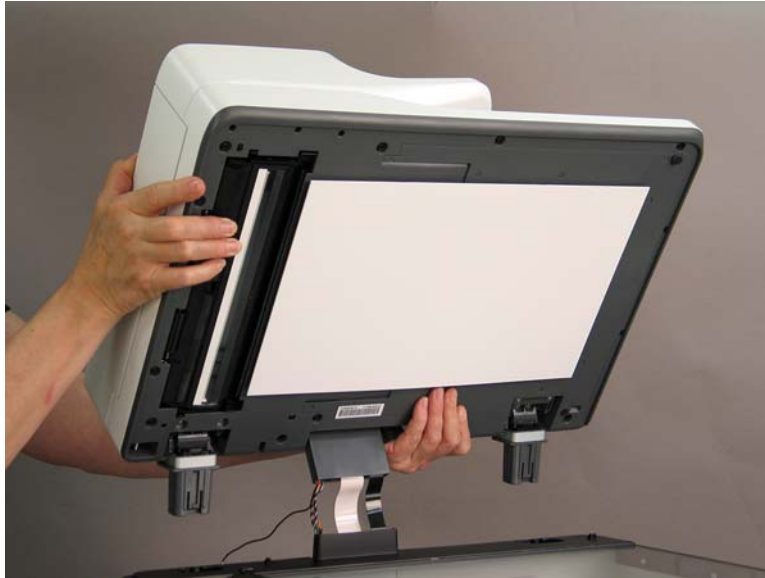
Figure 1-1195 Lift and remove the ADF
