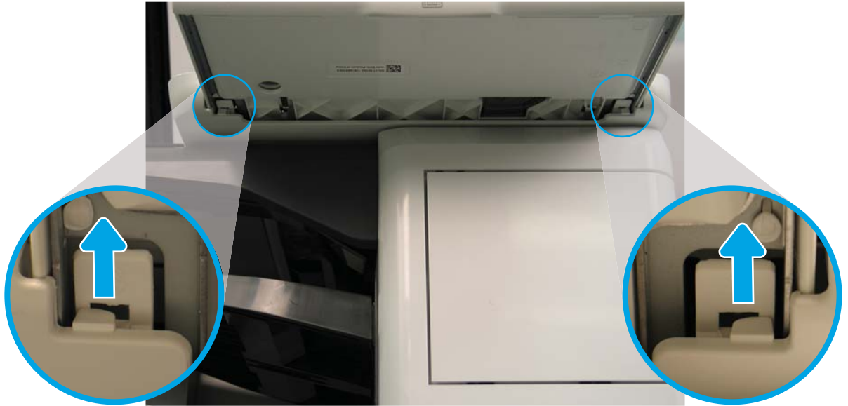
Figure 1-1095 Release two tabs
