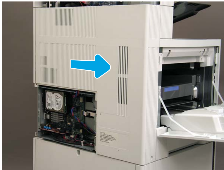
Figure 1-1112 Slide the rear cover
