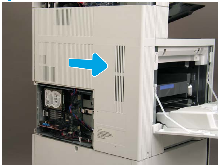
Figure 1-1220 Slide the rear cover
