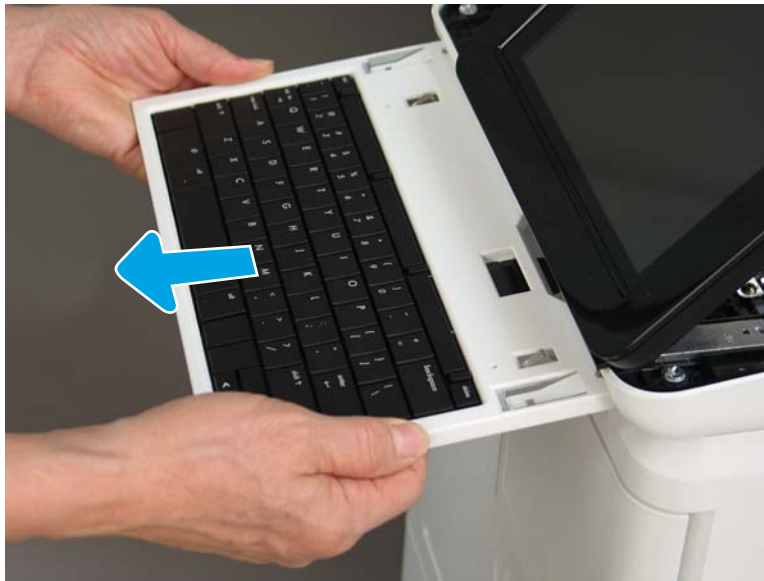
Figure 1-1183 Remove the keyboard
