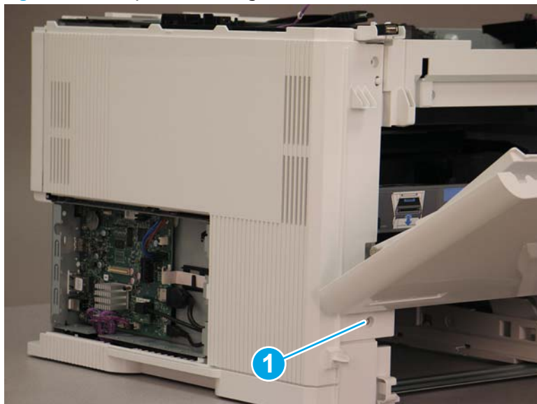
Figure 1-1992 Open the cartridge door and remove one screw
