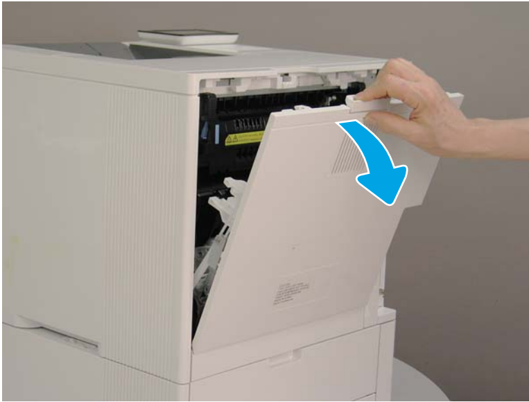
Figure 1-1775 Open the rear door
