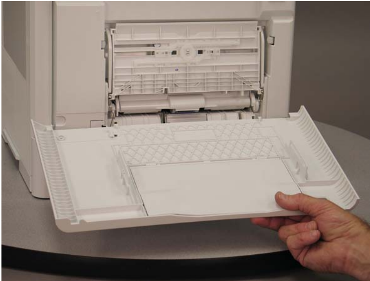
Figure 1-1898 Remove the MP cover
