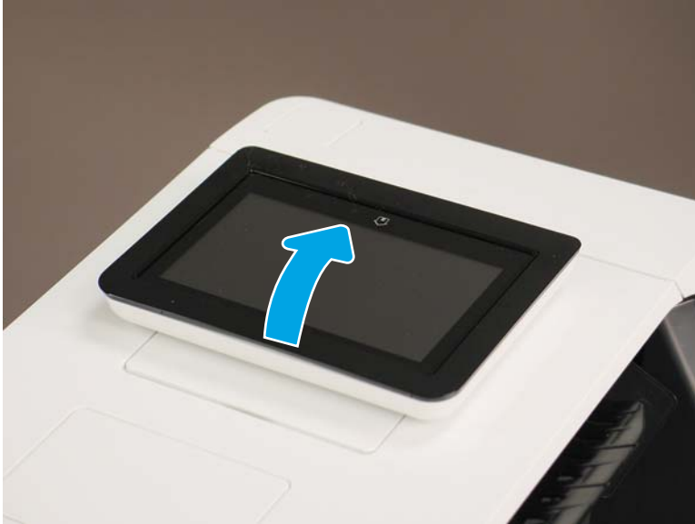
Figure 1-2029 Raise the control panel screen
