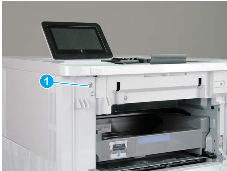
Figure 1-2020 Remove one screw
