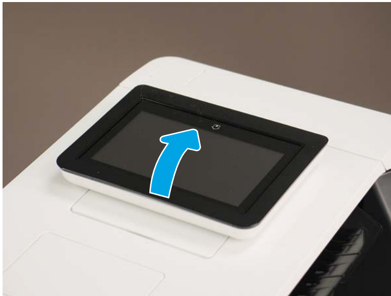
Figure 1-1957 Raise the control panel screen
