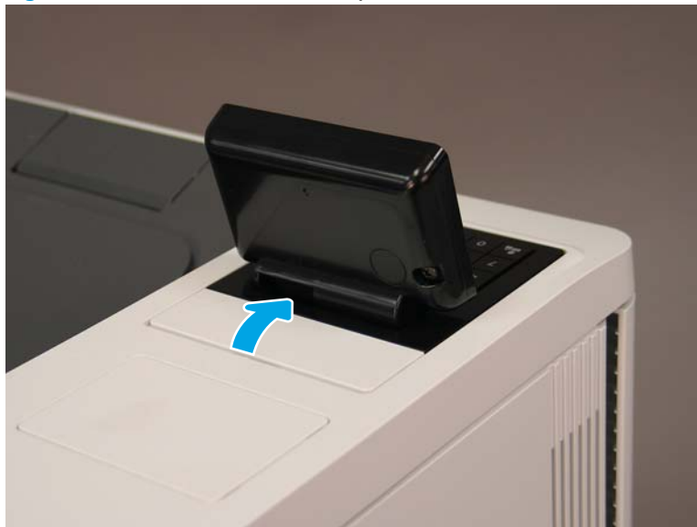
Figure 1-1709 Release the control panel cover and remove it
