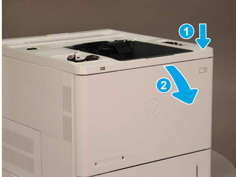
Figure 1-1840 Locate the tab and open the MP tray cover
