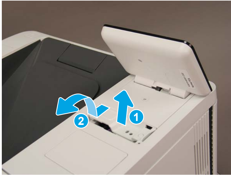
Figure 1-1960 Lift and release the control panel
