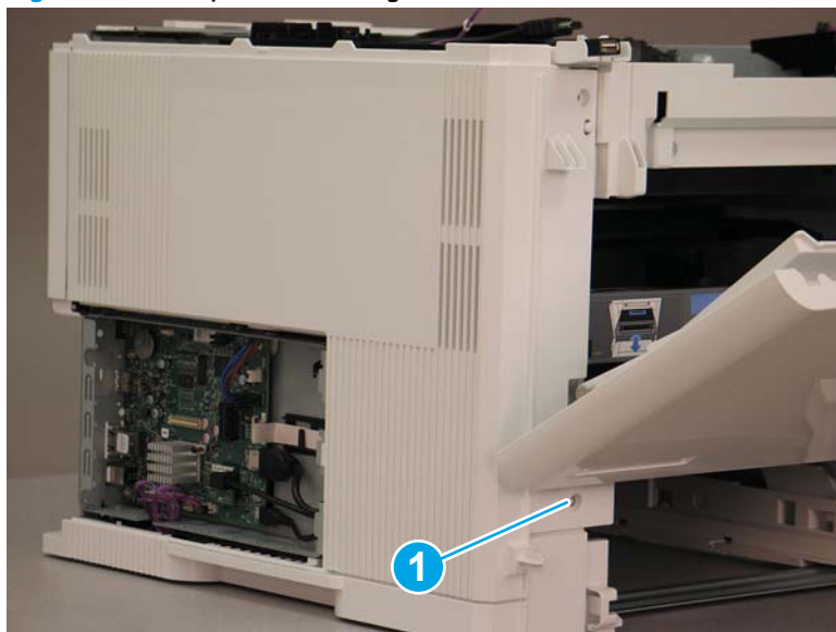
Figure 1-1820 Open the cartridge door and remove one screw
