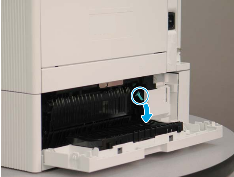
Figure 1-1779 Lower the access cover
