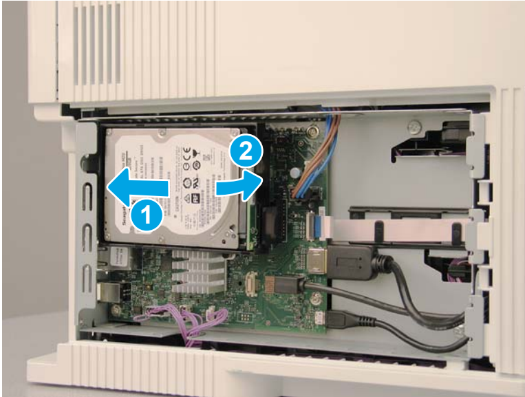
Figure 1-1759 Install the tab into the slot and rotate the connector end
