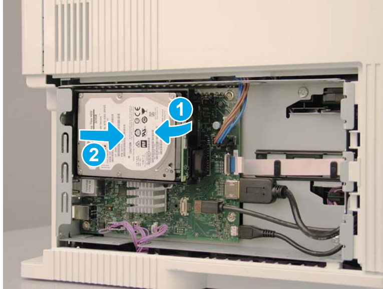
Figure 1-1754 Rotate the HDD away from the formatter and remove the HDD
