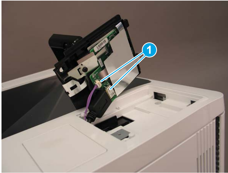
Figure 1-1712 Disconnect two connectors
