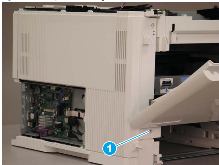
Figure 1-1845 Open the cartridge door and remove one screw
