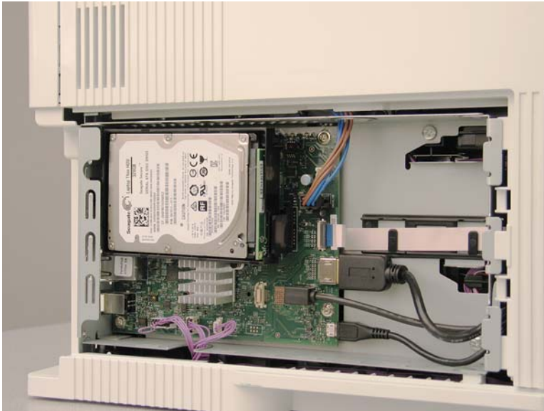
Figure 1-1764 Locate the space for installing the internal USB ports/AA module
