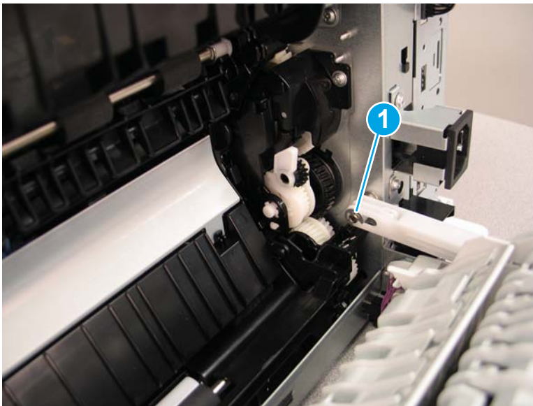
Figure 1-1937 Remove the e-ring
