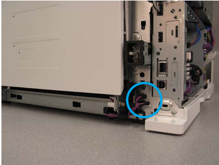
Figure 1-1935 Disconnect two connectors
