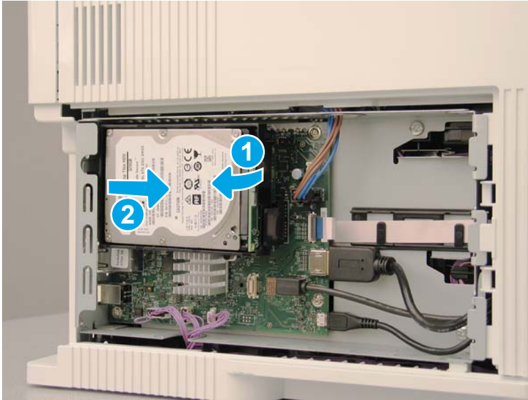
Figure 1-1742 Rotate the HDD away from the formatter and remove the HDD
