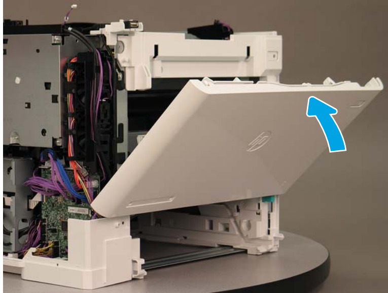
Figure 1-2175 Partially close the cartridge door
