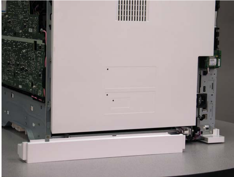
Figure 1-1951 Remove the rear lower cover
