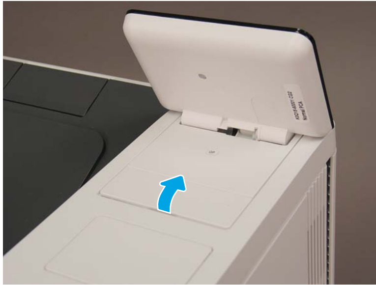
Figure 1-1906 Lift and remove the control panel cover
