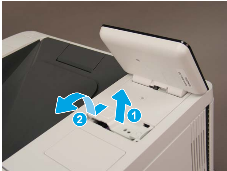
Figure 1-2184 Lift and release the control panel
