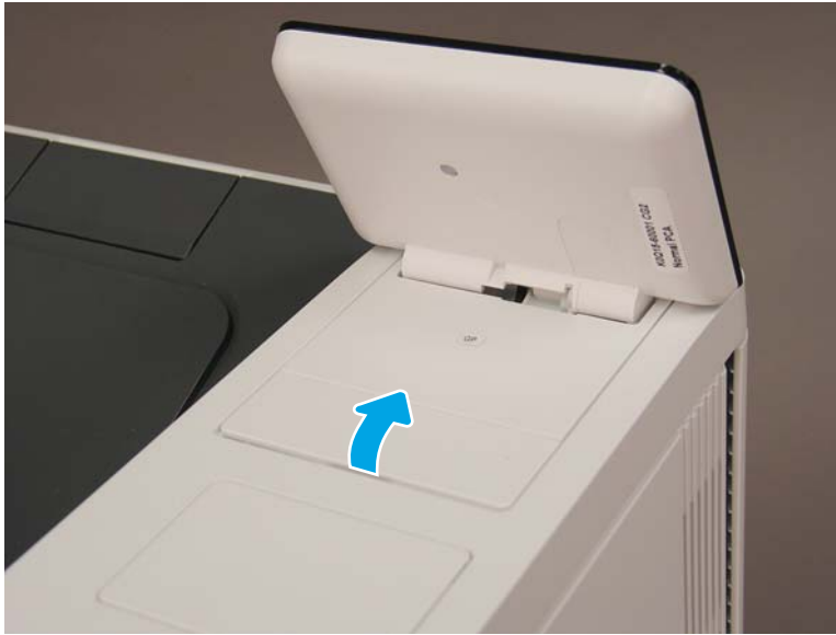
Figure 1-1958 Lift and remove the control panel cover
