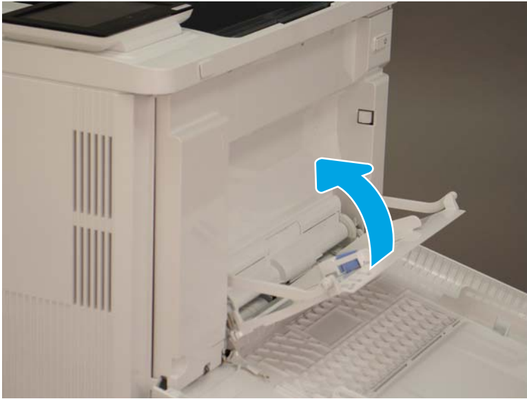
Figure 1-1879 Close the smaller MP tray assembly
