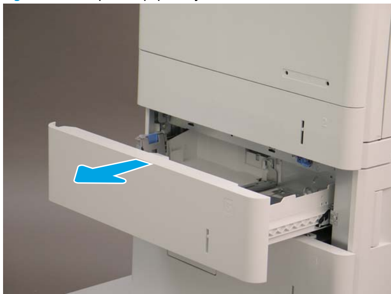
Figure 1-1773 Open the paper tray to locate the rollers
