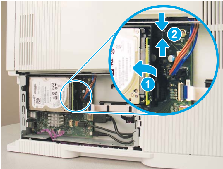
Figure 1-1753 Release the locking connector and release the HDD retainer
