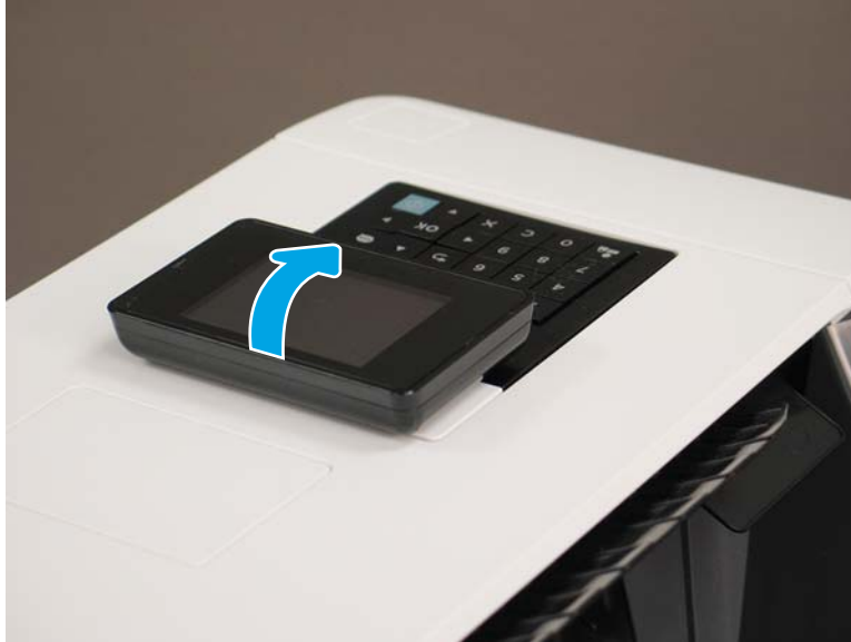
Figure 1-1708 Raise the control panel screen
