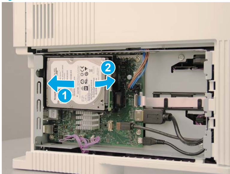
Figure 1-1744 Install the tab into the slot and rotate the connector end
