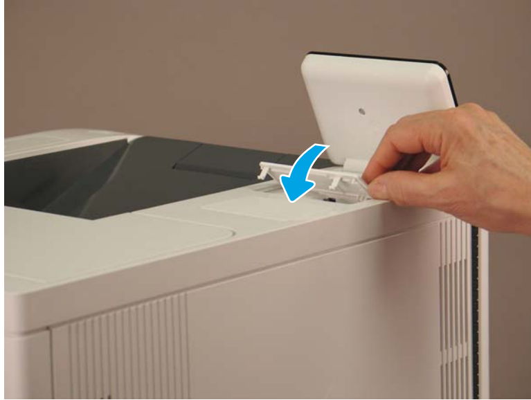
Figure 1-1707 Align the control panel cover and pivot down to install it
