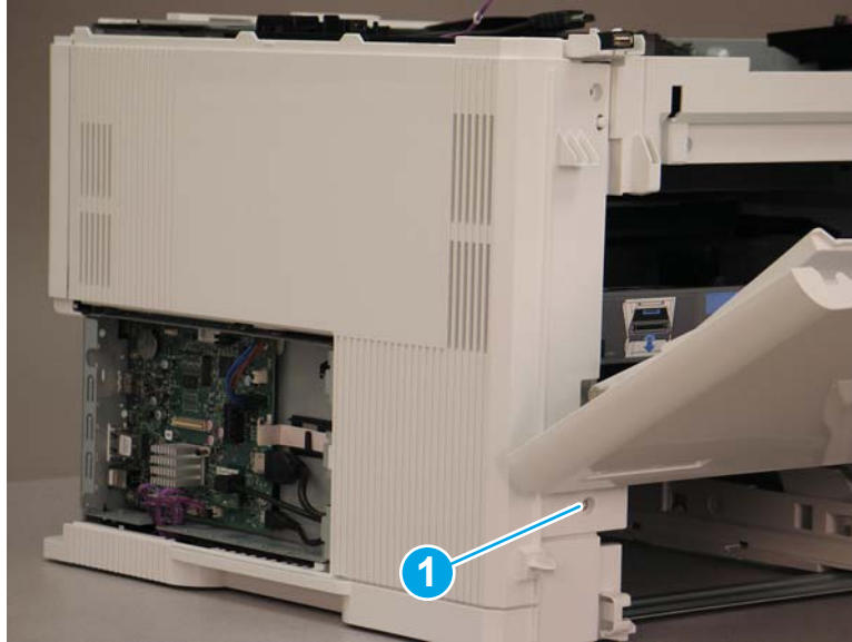
Figure 1-2171 Open the cartridge door and remove one screw
