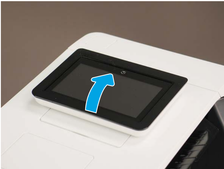
Figure 1-1976 Raise the control panel screen
