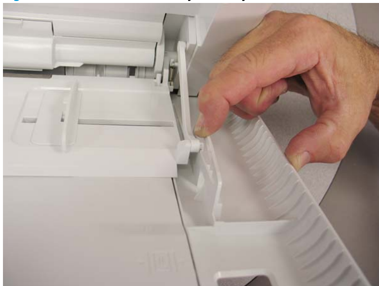
Figure 1-1878 Release the MP tray assembly lift arms from the MP cover
