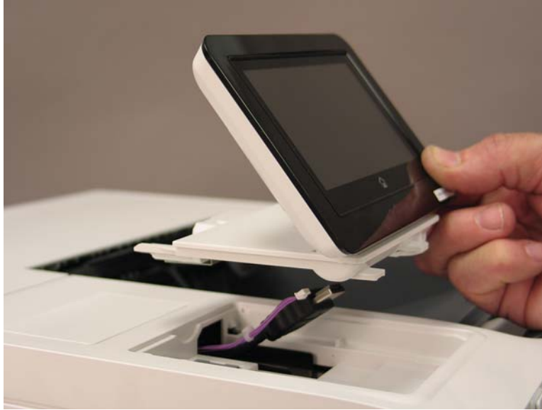
Figure 1-1981 Remove the control panel
