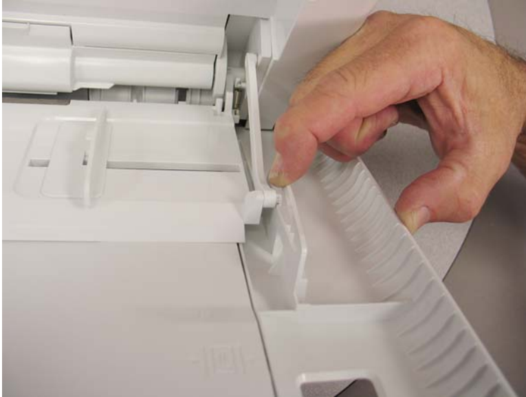
Figure 1-1894 Release the MP tray assembly lift arms from the MP cover
