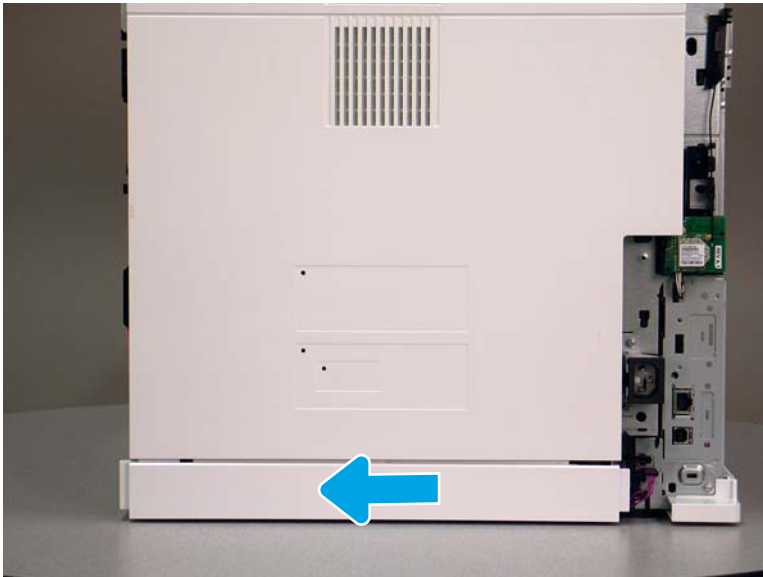
Figure 1-1950 Slide the rear lower cover
