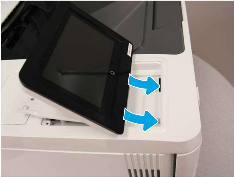
Figure 1-1705 Install the control panel tabs into the printer slots
