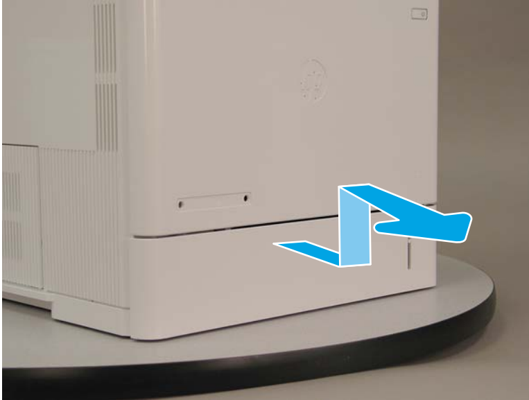
Figure 1-1904 Open and remove the cassette tray 2
