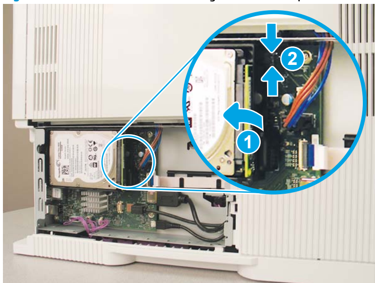
Figure 1-1741 Release the HDD locking connector and pinch the retainer to release it
