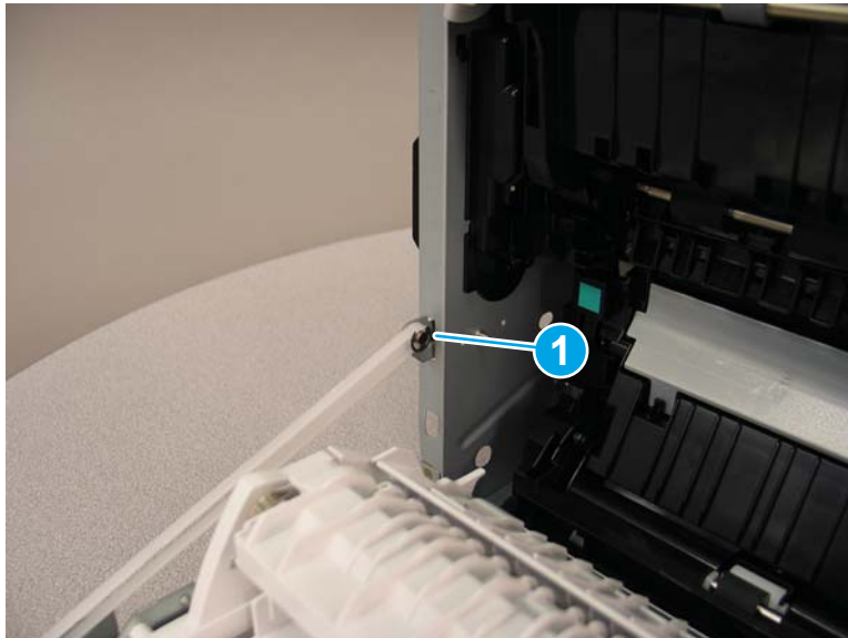
Figure 1-1939 Remove the e-ring
