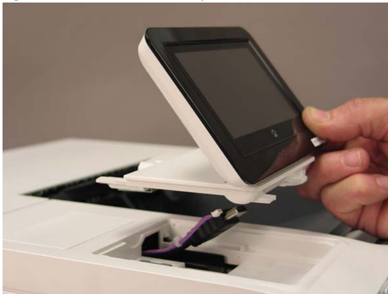
Figure 1-2004 Remove the control panel
