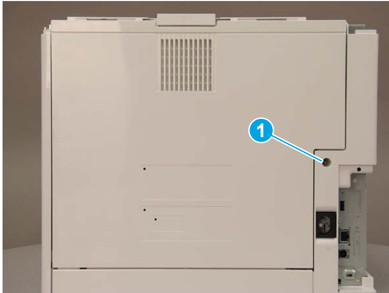
Figure 1-2108 Remove one screw
