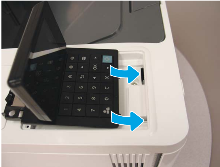
Figure 1-1715 Install the control panel tabs into the printer slots
