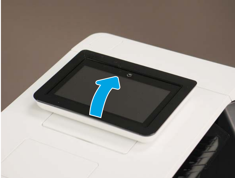
Figure 1-2097 Raise the control panel screen
