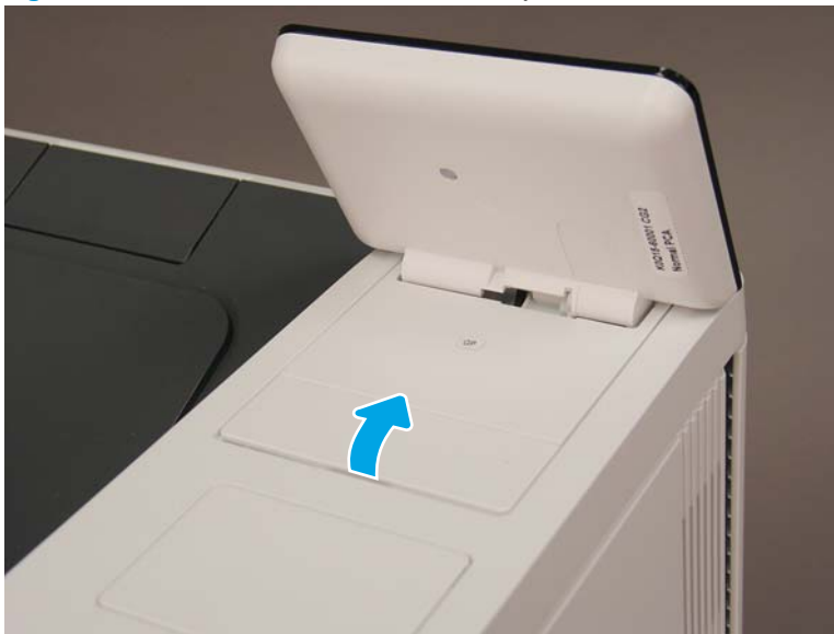
Figure 1-1864 Lift and remove the control panel cover
