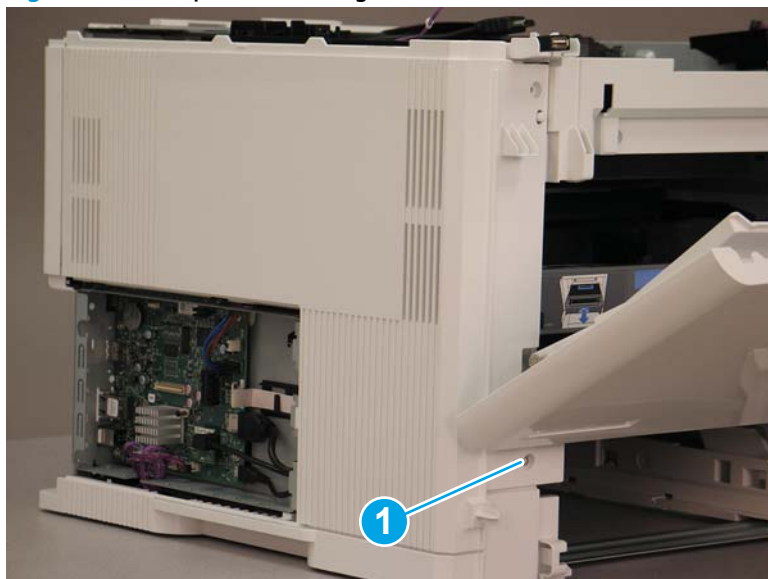
Figure 1-1953 Open the cartridge door and remove one screw
