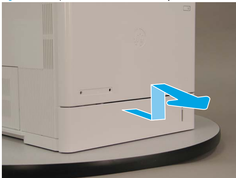
Figure 1-1844 Open and remove the cassette tray 2
