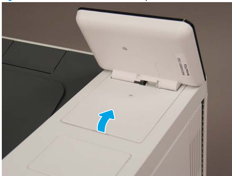
Figure 1-2000 Lift and remove the control panel cover
