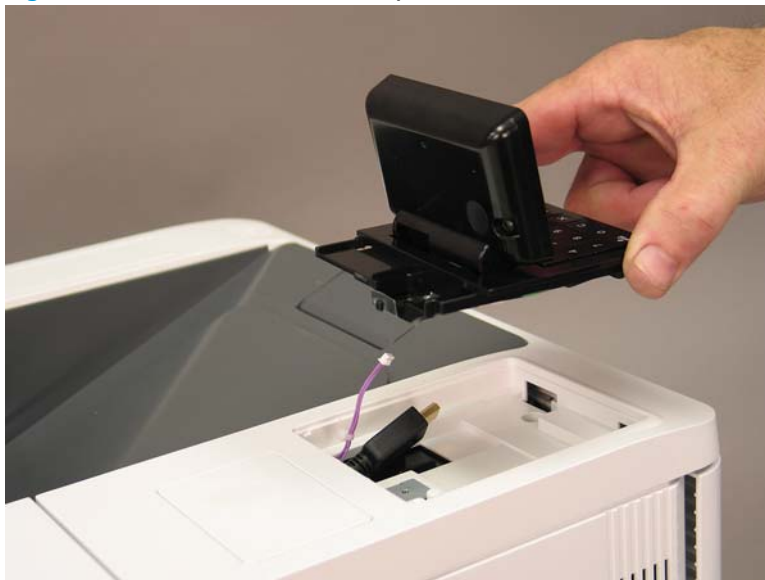
Figure 1-1713 Remove the control panel
