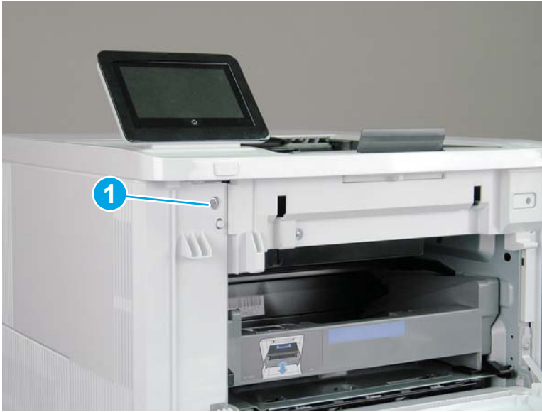
Figure 1-1816 Remove one screw
