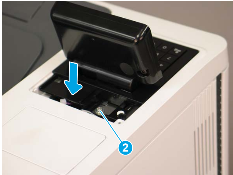
Figure 1-1716 Lower the control panel and install one thumbscrew
