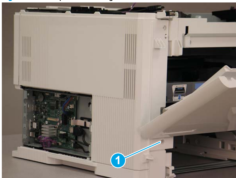
Figure 1-1815 Open the cartridge door and remove one screw
