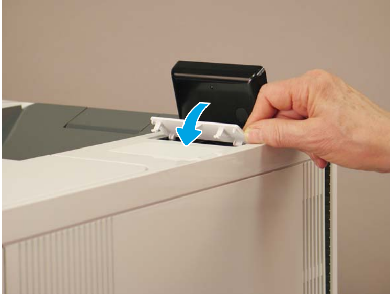
Figure 1-1717 Align the control panel cover and pivot down to install it
