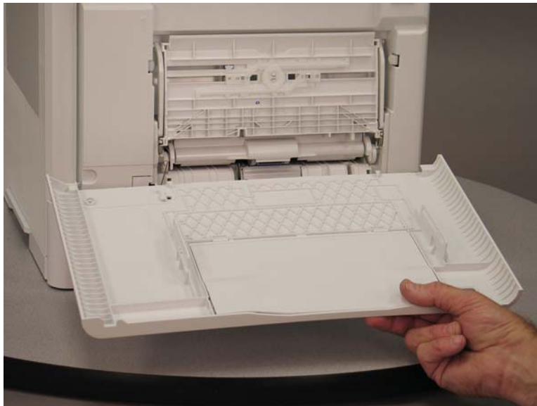
Figure 1-1882 Remove the MP cover
