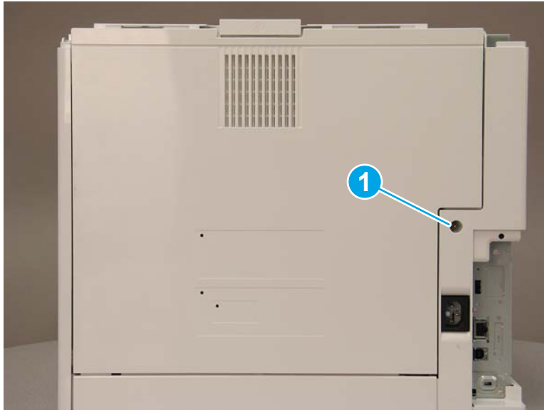
Figure 1-2040 Remove one screw
