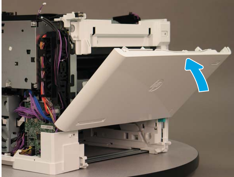
Figure 1-2023 Partially close the cartridge door
