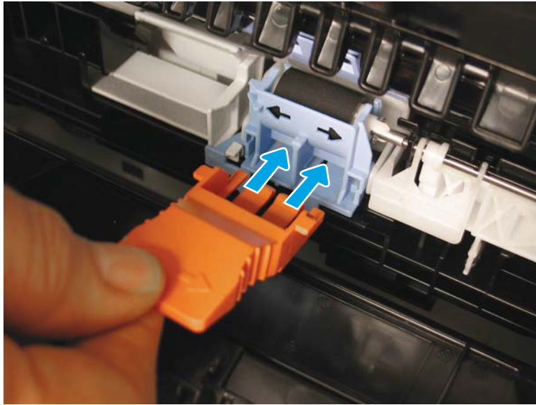
Figure 1-1782 Install the orange tool in the separation roller
