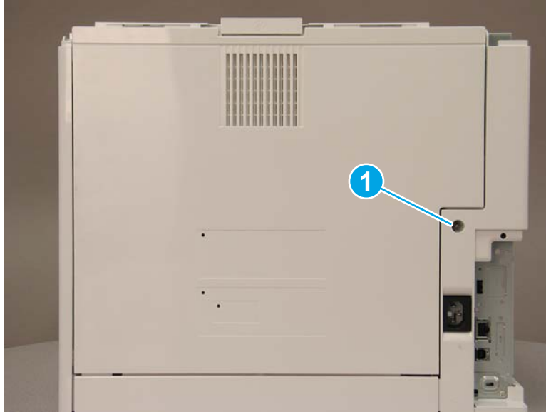
Figure 1-2496 Remove one screw
