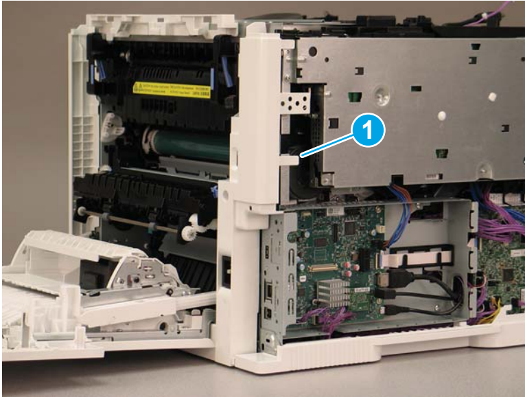
Figure 1-2288 Release the tab and remove the inlet cover
