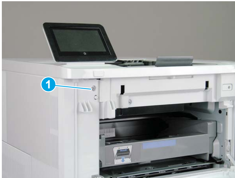
Figure 1-2442 Remove one screw
