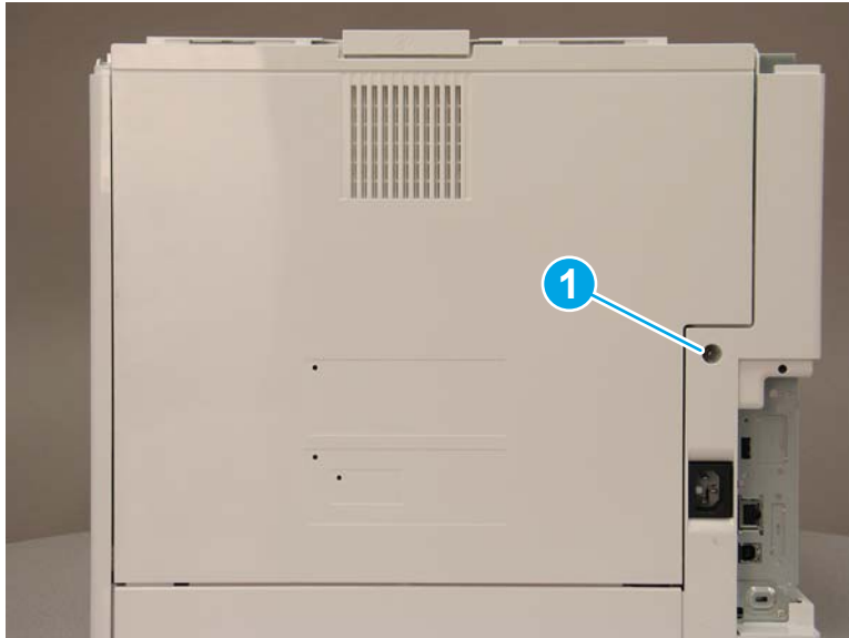
Figure 1-2192 Remove one screw
