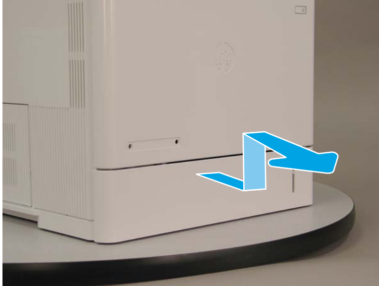
Figure 1-2471 Open and remove the cassette tray 2
