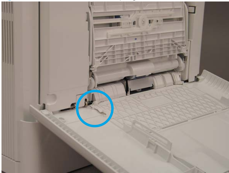
Figure 1-2451 Disconnect the left spring
