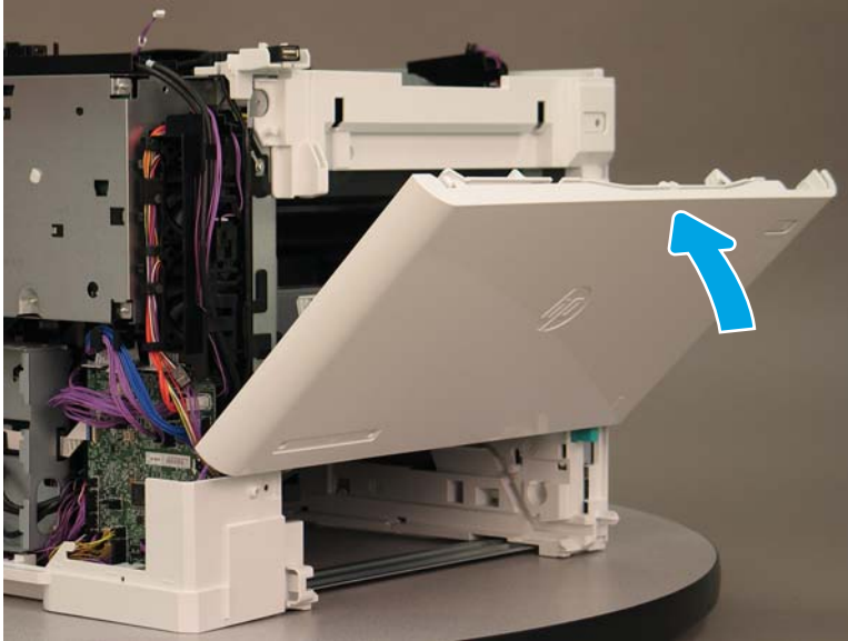
Figure 1-2323 Partially close the cartridge door
