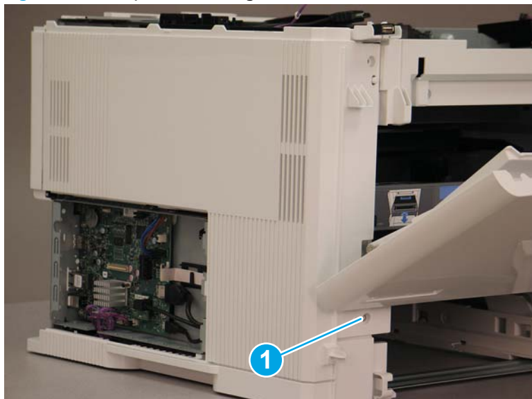
Figure 1-2464 Open the cartridge door and remove one screw
