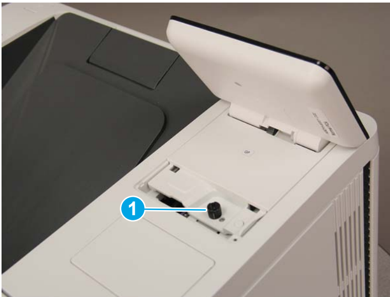
Figure 1-2479 Remove one thumbscrew
