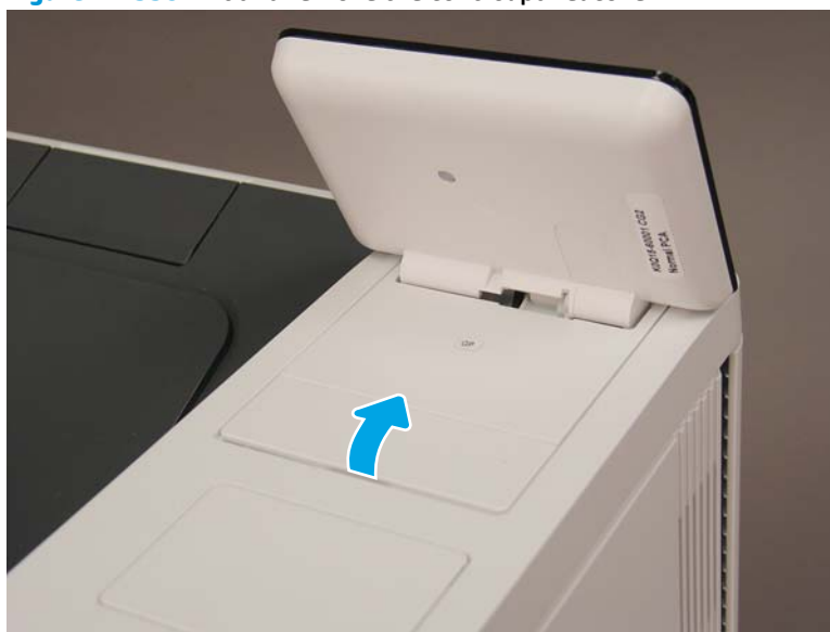
Figure 1-2330 Lift and remove the control panel cover
