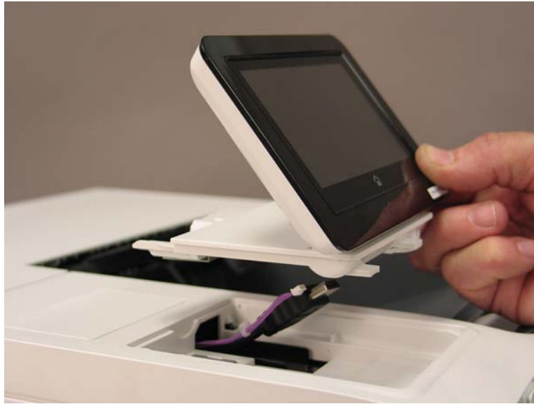
Figure 1-2262 Remove the control panel
