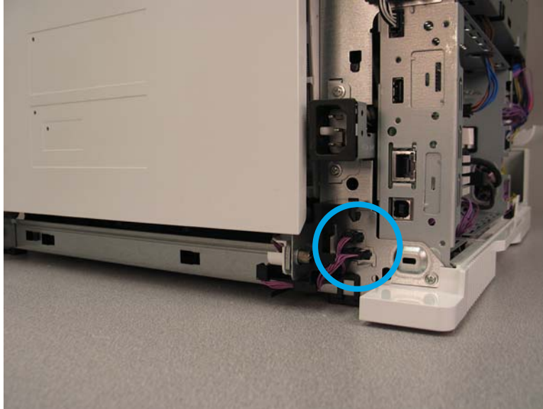
Figure 1-2278 Disconnect two connectors
