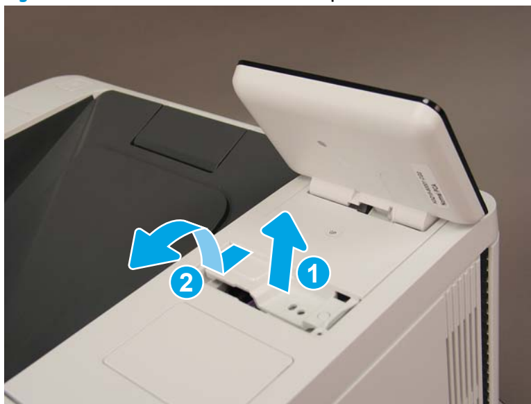
Figure 1-2219 Lift and release the control panel
