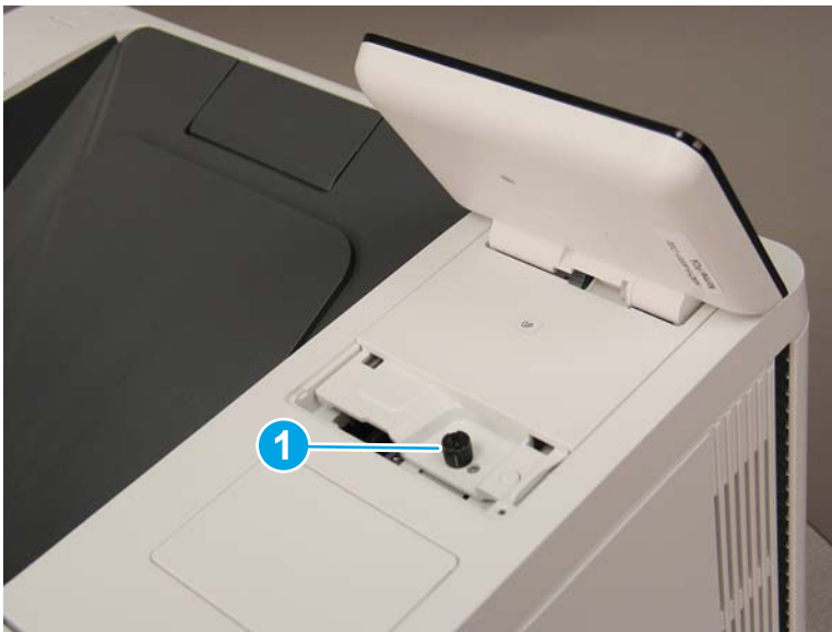
Figure 1-2218 Remove one thumbscrew
