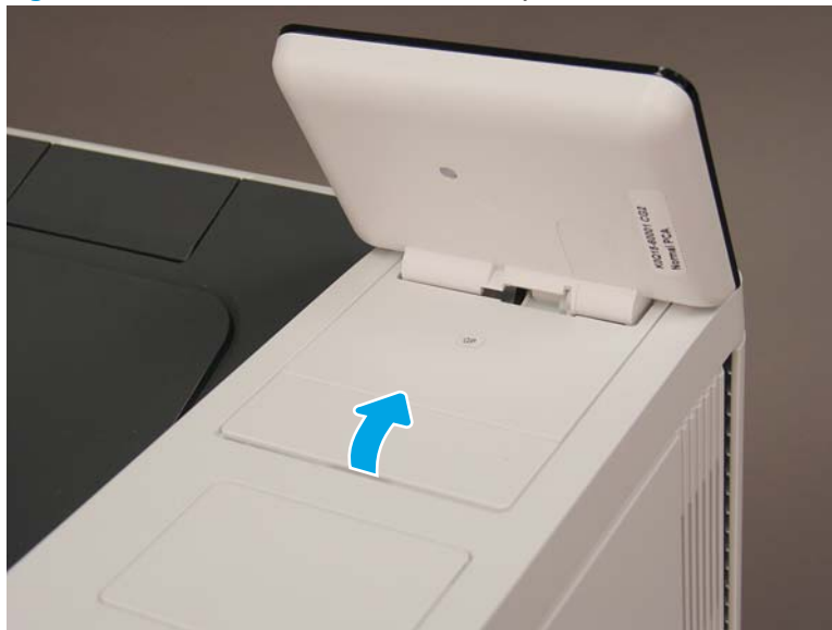
Figure 1-2390 Lift and remove the control panel cover
