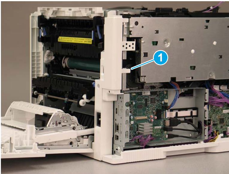
Figure 1-2498 Release the tab and remove the inlet cover
