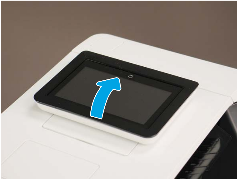
Figure 1-2257 Raise the control panel screen
