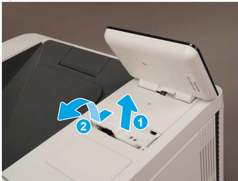
Figure 1-2480 Lift and release the control panel
