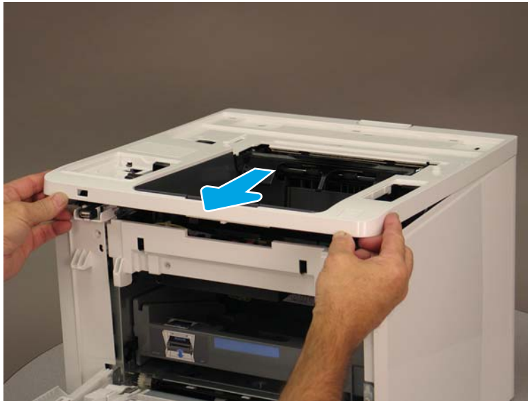
Figure 1-2228 Slide the top cover
