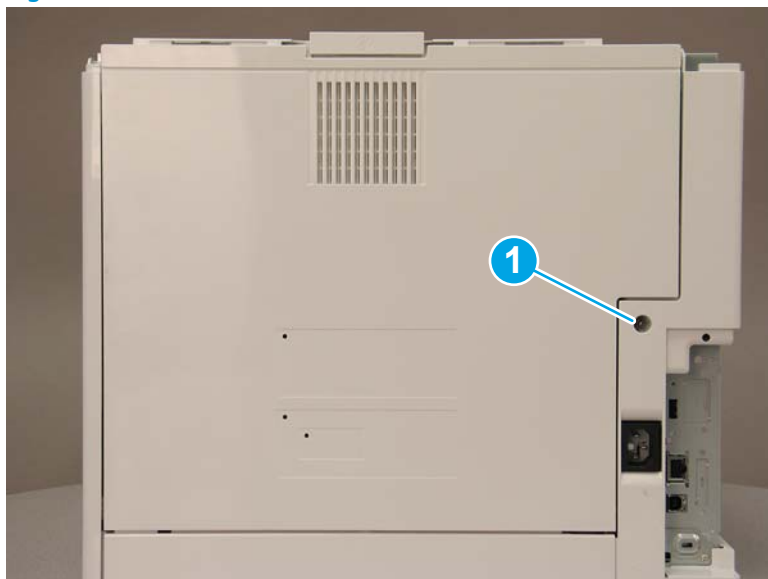
Figure 1-2240 Remove one screw
