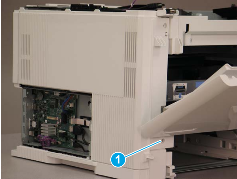
Figure 1-2379 Open the cartridge door and remove one screw
