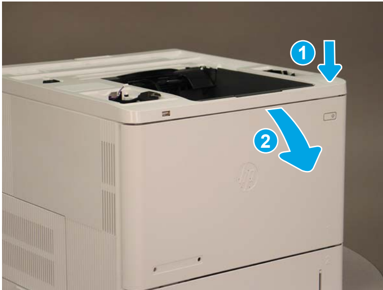
Figure 1-2336 Locate the tab and open the MP tray cover
