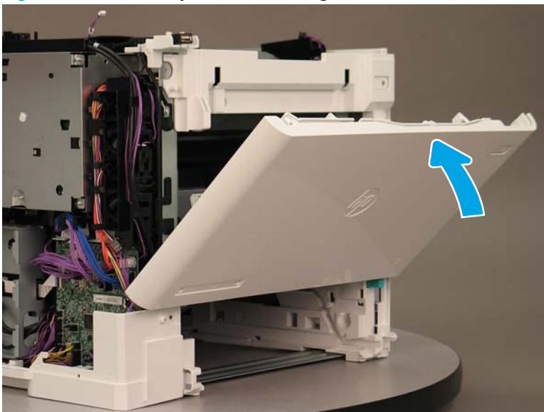
Figure 1-2445 Partially close the cartridge door
