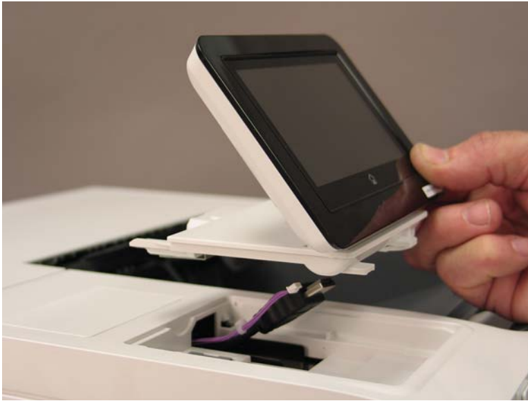
Figure 1-2482 Remove the control panel
