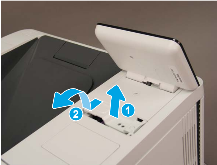
Figure 1-2260 Lift and release the control panel
