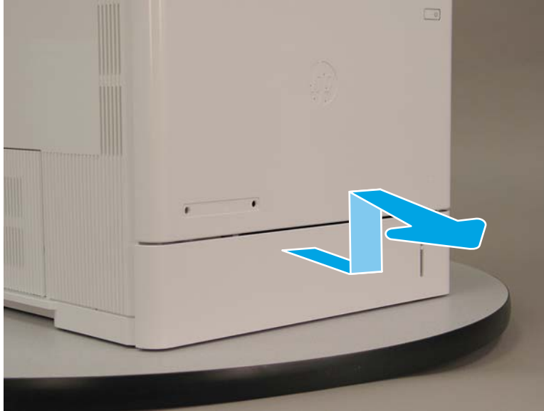
Figure 1-2502 Open and remove the cassette tray 2
