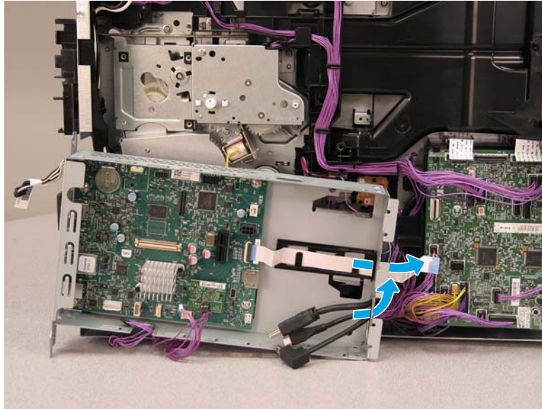
Figure 1-2251 Pull one cable and the FFC through the formatter cage
