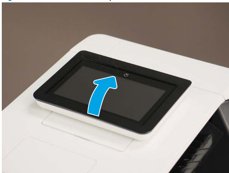
Figure 1-2477 Raise the control panel screen
