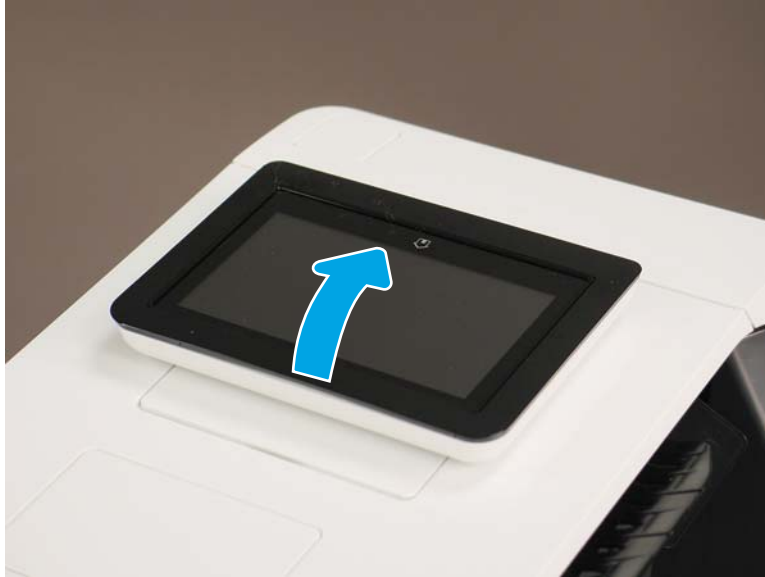
Figure 1-2389 Raise the control panel screen
