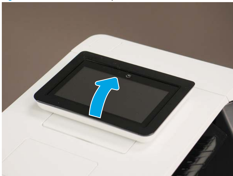
Figure 1-2329 Raise the control panel screen
