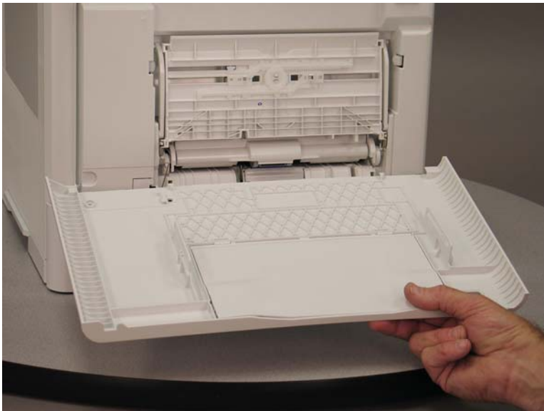
Figure 1-2453 Remove the MP cover
