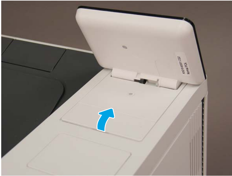
Figure 1-2478 Lift and remove the control panel cover
