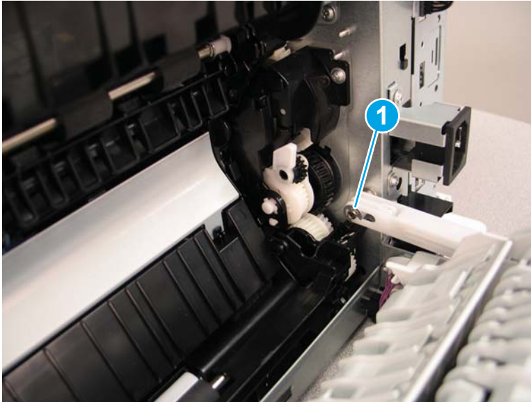
Figure 1-2280 Remove the e-ring
