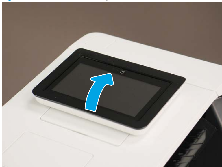
Figure 1-2216 Raise the control panel screen
