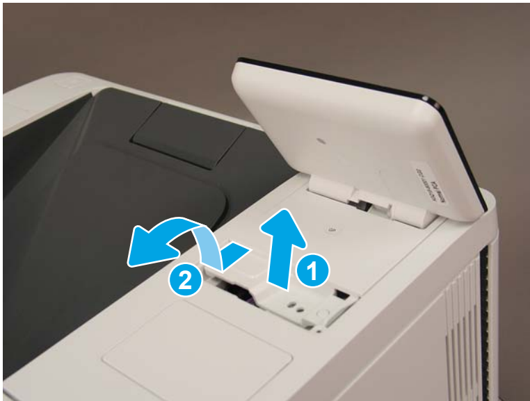
Figure 1-2332 Lift and release the control panel
