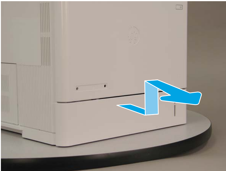
Figure 1-2491 Open and remove the cassette tray 2
