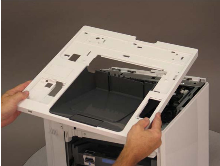
Figure 1-2399 Lift and remove the top cover
