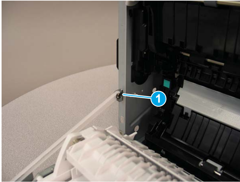
Figure 1-2282 Remove the e-ring
