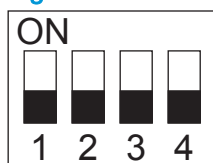
Figure 1-1057 SW601 sensor adjustment settings
