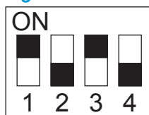
Figure 1-1059 SW601 sensor adjustment settings
