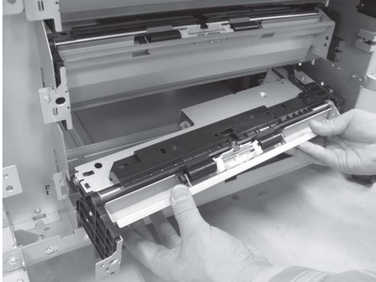
Figure 1-611 Remove the 3x500 Tray 5 pickup assembly (3 of 3)
