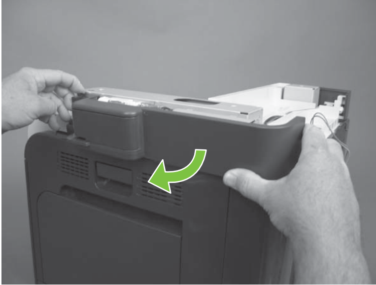
Figure 6-117 Remove the front stapler cover and right-side stapler cover (10 of 13)
