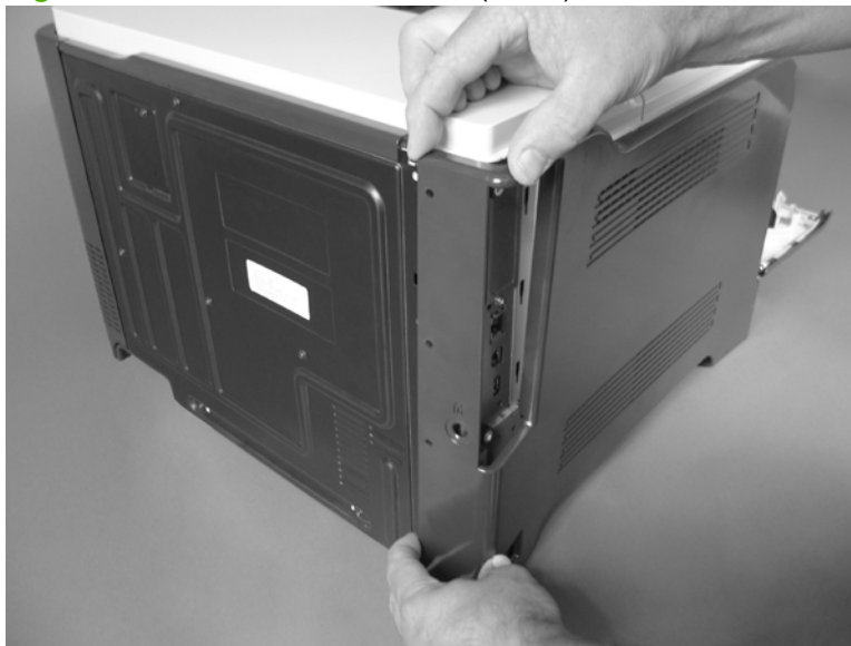
Figure 6-81 Remove the left cover (2 of 5)
