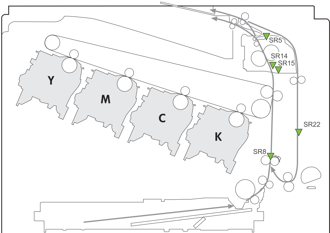
Figure 5-43 Jam detection sensors
