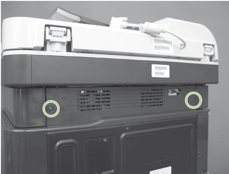
Figure 6-86 Remove the rear-upper cover (2 of 4)
