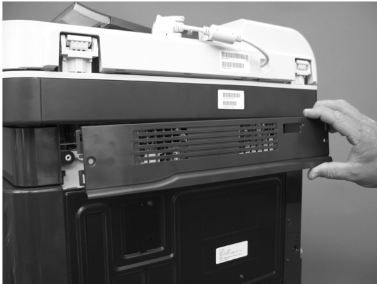
Figure 6-88 Remove the rear-upper cover (4 of 4)
