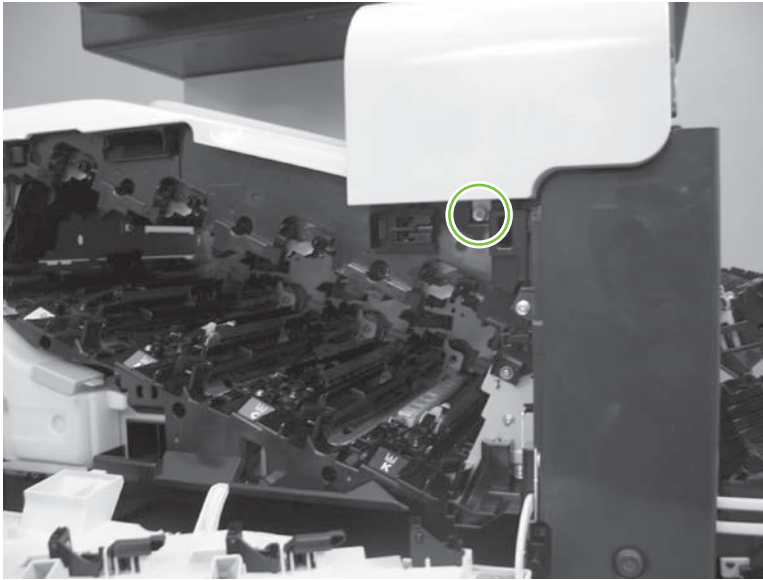
Figure 6-67 Remove the front-upper cover (3 of 4)
