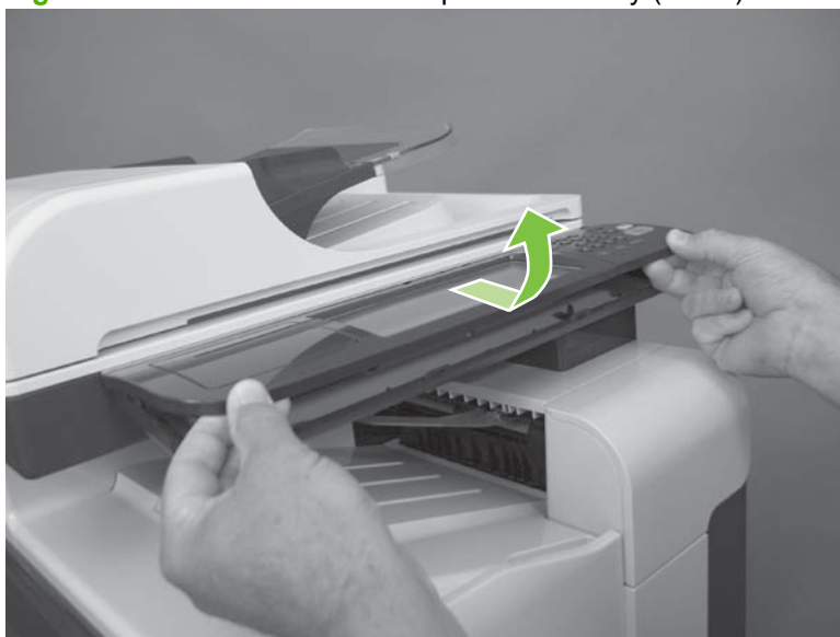
Figure 6-59 Remove the control-panel assembly (2 of 3)
