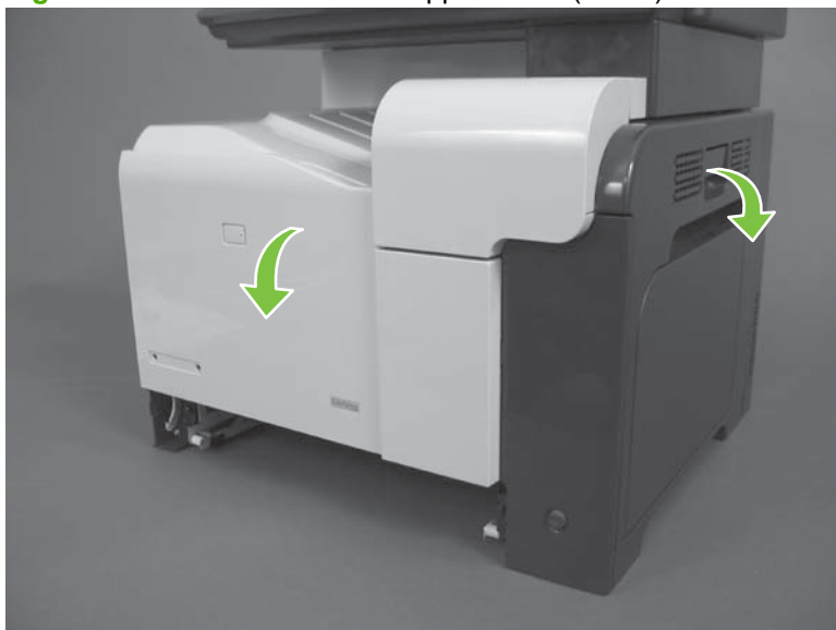
Figure 6-65 Remove the front-upper cover (1 of 4)
