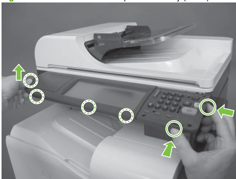
Figure 6-58 Remove the control-panel assembly (1 of 3)
