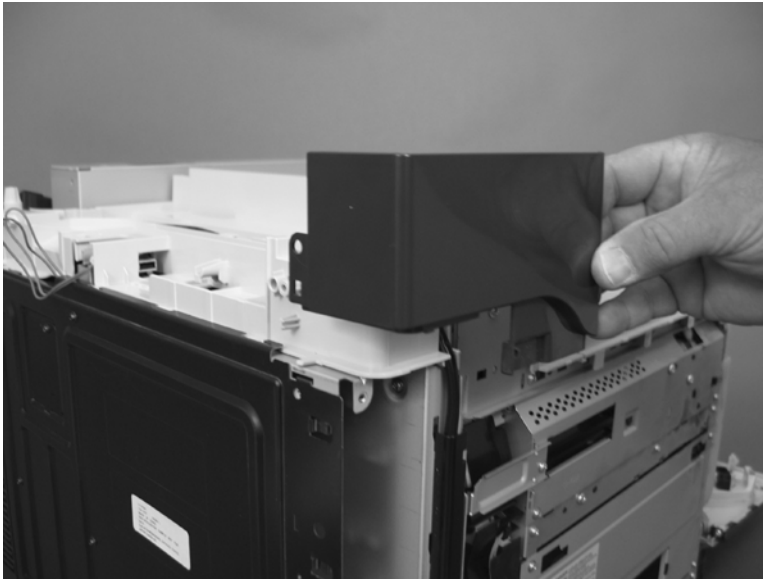
Figure 6-107 Remove the left-upper cover (2 of 2)
