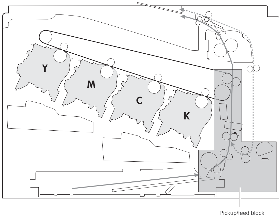
Figure 5-30 Pickup and feed unit
