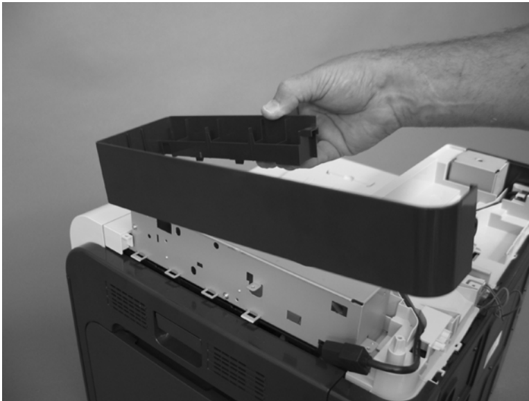
Figure 6-128 Remove the right-top cover (5 of 5)
