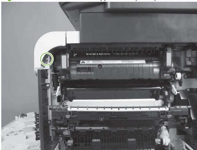
Figure 6-66 Remove the front-upper cover (2 of 4)
