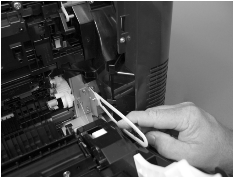
Figure 6-72 Remove the right-door assembly (4 of 8)
