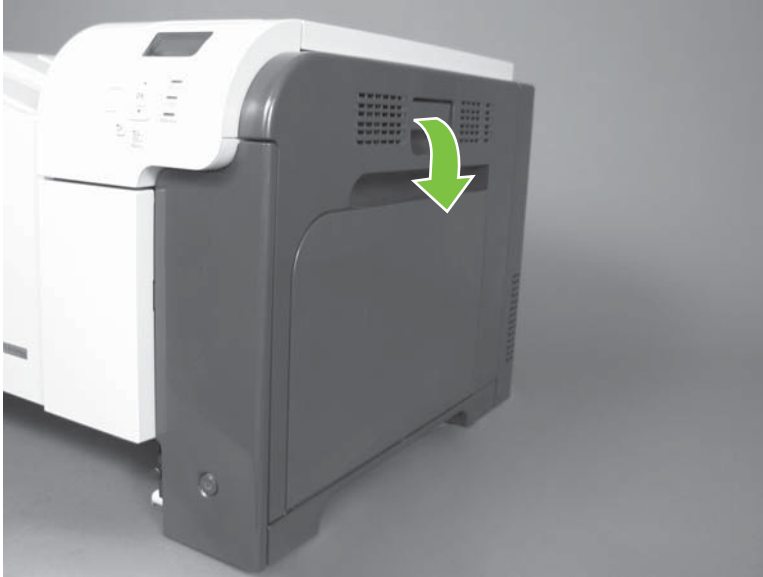
Figure 6-24 Remove the fuser (1 of 2)
