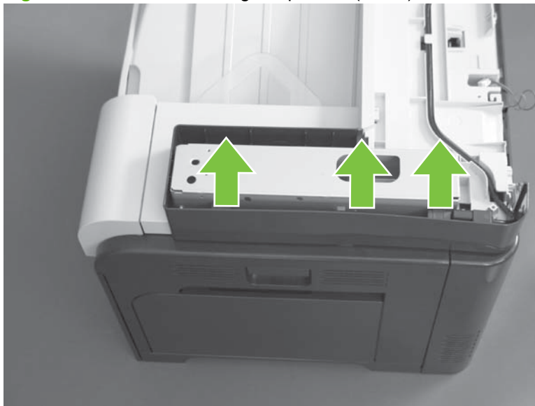
Figure 6-126 Remove the right-top cover (3 of 5)
