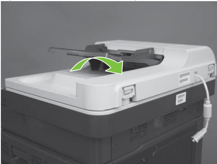
Figure 6-47 Remove the ADF assembly (2 of 4)
