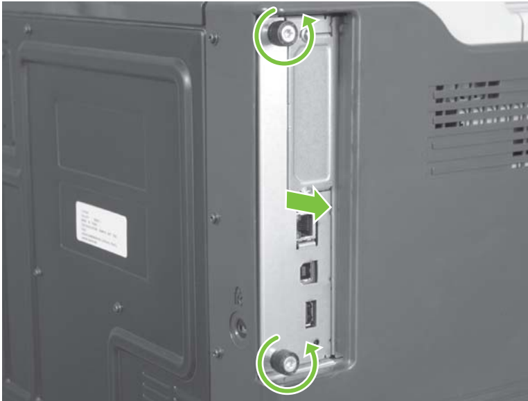
Figure 6-14 Remove the formatter
