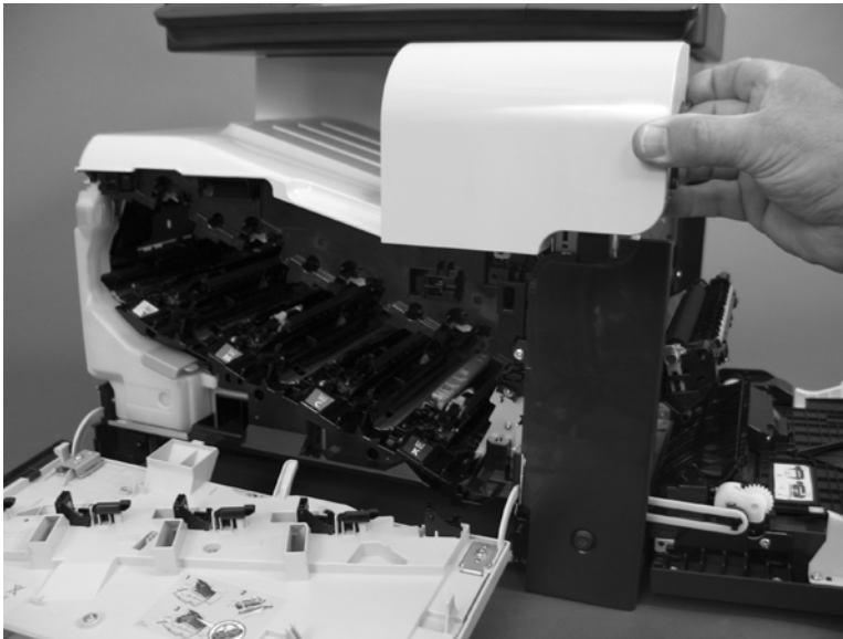
Figure 6-68 Remove the front-upper cover (4 of 4)
