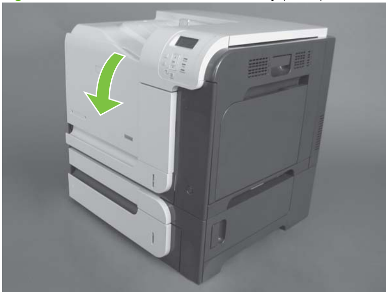
Figure 6-44 Remove the front-door assembly (1 of 2)
