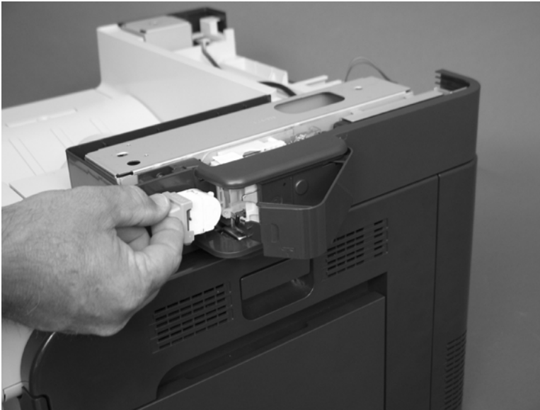
Figure 6-7 Remove the stapler cartridge
