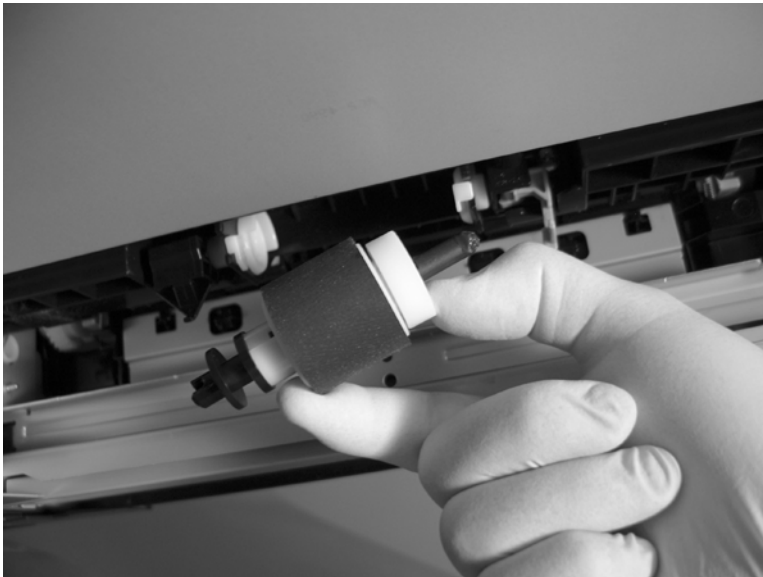
Figure 6-29 Remove the pickup roller (Tray 2) (4 of 4)
