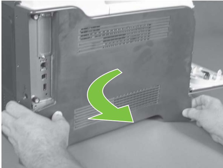
Figure 6-84 Remove the left cover (5 of 5)
